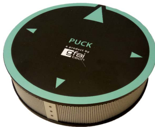
Figure 1 – Array of 16 microphones disposed in a circumference of 20 cm diameter (PUCK)
