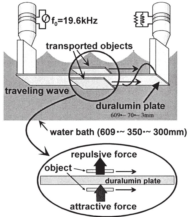
Fig.6. Underwater transportation system using a traveling wave
