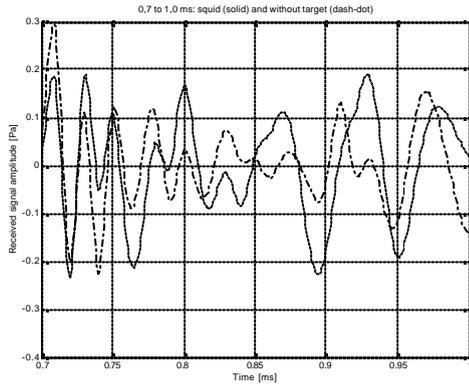
Fig.5. Received sound pressures from 0.7 to 1.0 ms lags without a target (dash-dot) and with a squid target (solid).
