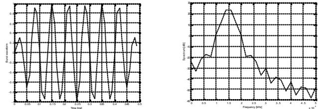
Fig.3. Transmitted burst and waveform spectrum (logarithmic scale, arbitrary reference)
