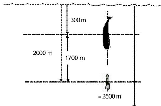
The sperm whale click source level of 230 dB<sub>peak</sub> and the diameter of the modelled circular piston radiator of 0.8 m, as given by Mohl et al [8] were used. The *Loligo vulgaris* specimen with a target strength of -36.3 dB used for the measurements was also used as the imagined target in these simulations. The
