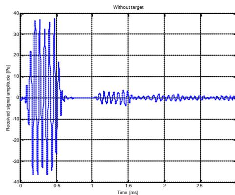
Fig. 4. Received waveform converted to pressure, no target present
