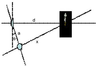
Fig.2. Measurement setup:  $d = 50$  cm,  $a = 12$  cm,  $q = 15^\circ$
