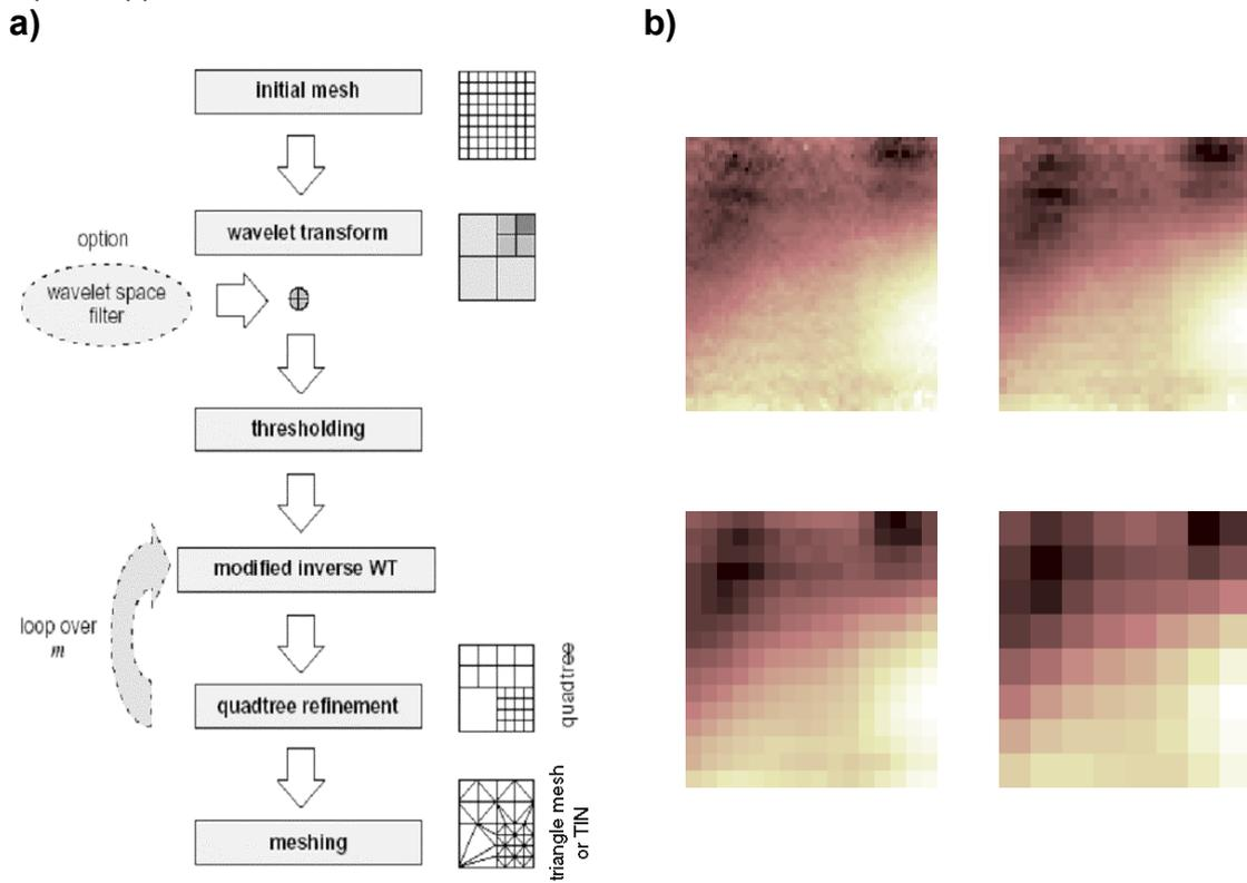
Fig.2. Algorithm of efficient triangular surface approximation using wavelet and quadtree data structures meshing (left). Level of detail (LOD) representation of sea bottom image (right).
