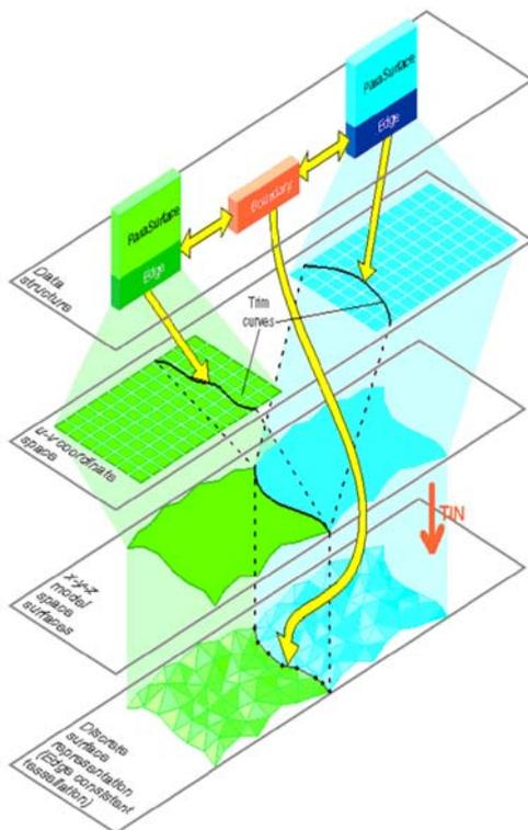
Fig.1.Spline model of sonar data for 3<sup>D</sup> imaging of seafloor accord.[4].
