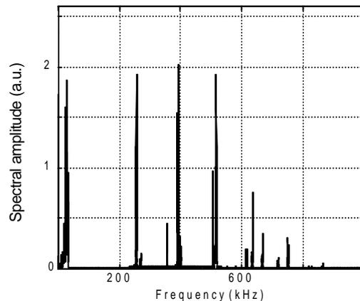
Figure 5. Frequency domain. Squared packing excited with a shear impulsion. 20 kg applied load.
