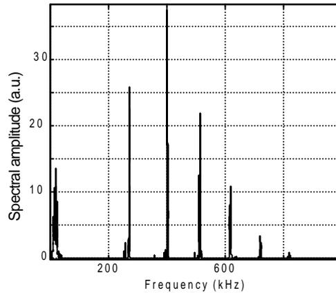
Figure 3. Frequency domain. Squared packing excited with a longitudinal impulsion. 60 kg applied load.
