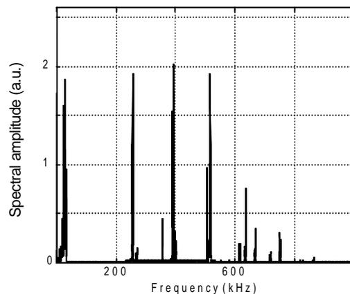
Figure 5. Frequency domain. Squared packing excited with a shear impulsion. 20 kg applied load.
