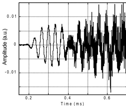
Figure 4. Time domain. Squared packing excited with a shear impulsion. 20 kg applied load.
