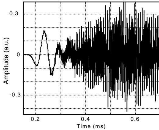
Figure 2. Time domain. Squared packing excited with a longitudinal impulsion. 60 kg applied load.
