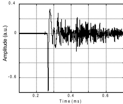
Figure 8. Time domain. Glass beads granular medium.
