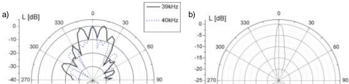
Fig.5. Directional characteristic of: a) the primary waves sources, b) the parametric source for the frequency of 1 kHz.
