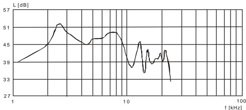
Fig.8. Frequency characteristic of the parametric source from primary waves with frequency 160 and 159 kHz.
