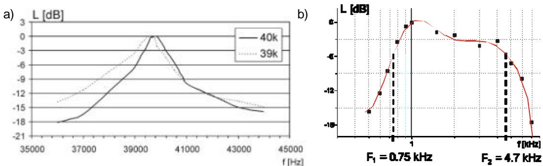
Fig.6. Frequency characteristic of: a) the primary waves sources, b) the parametric source.
