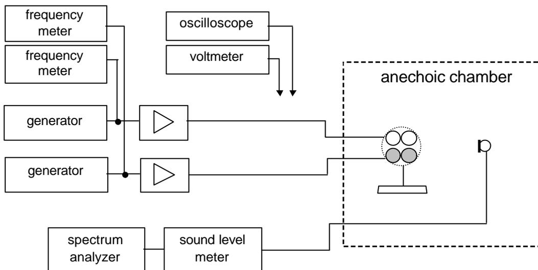
Fig.3. Measurement set-up for the examination of parametric sources.
