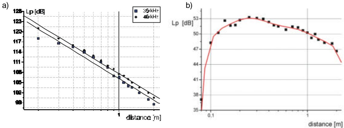
Fig.4. Dependence of the level of acoustic pressure of: a) the primary waves 40 kHz and 39 kHz on the distance from the source, b) the differential wave on the distance from the source.
