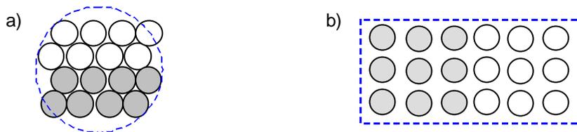
Fig.2. Distribution of transducers in the matrix in the band of: a) 40 kHz, b) 160 kHz.
