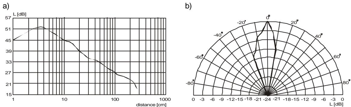
Fig.7. Measurement results of parametric wave from primary waves with frequency 160 and 159 kHz: a) level of the differential wave pressure in the distance function, b) directional characteristic of the parametric source measured at the distance of 3 m from the matrix.
