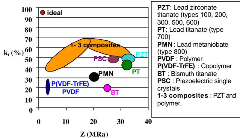
Figure 1 : Electromechanical coupling factor in thickness mode ( $k_t$ ) versus the acoustical impedance for different piezoelectric materials.
