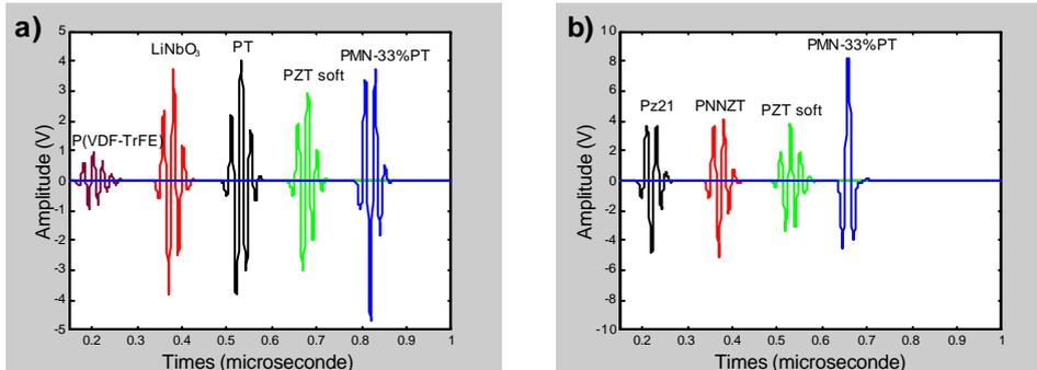
Figure 2 : Impulse responses of the two simulations (a- single element transducer, b one element of a 2D array) for a 60 V amplitude and 20ns duration pulse.
