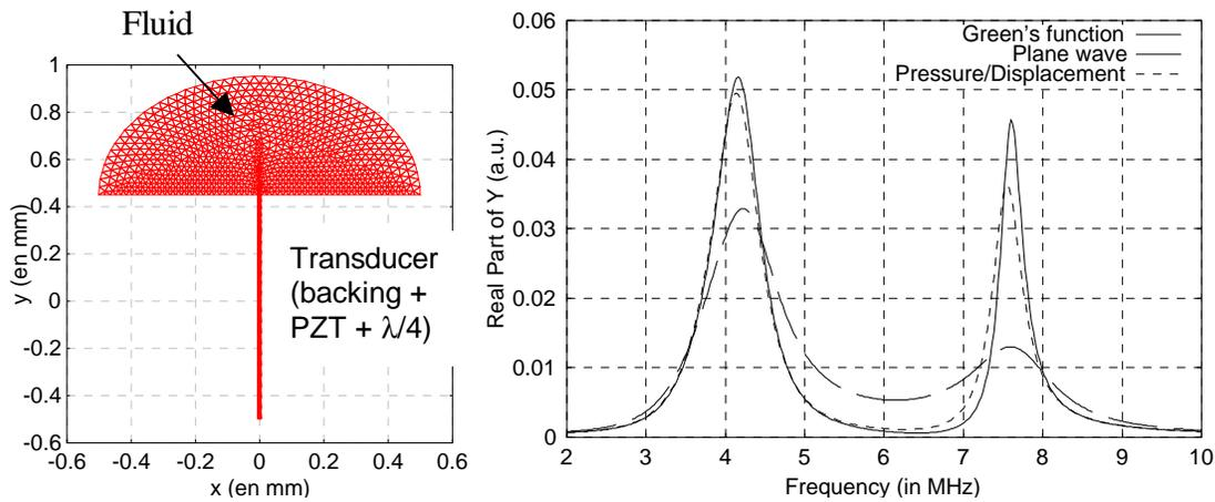
fig.6 Comparison between the three proposed approaches for addressing fluid/solid interaction
