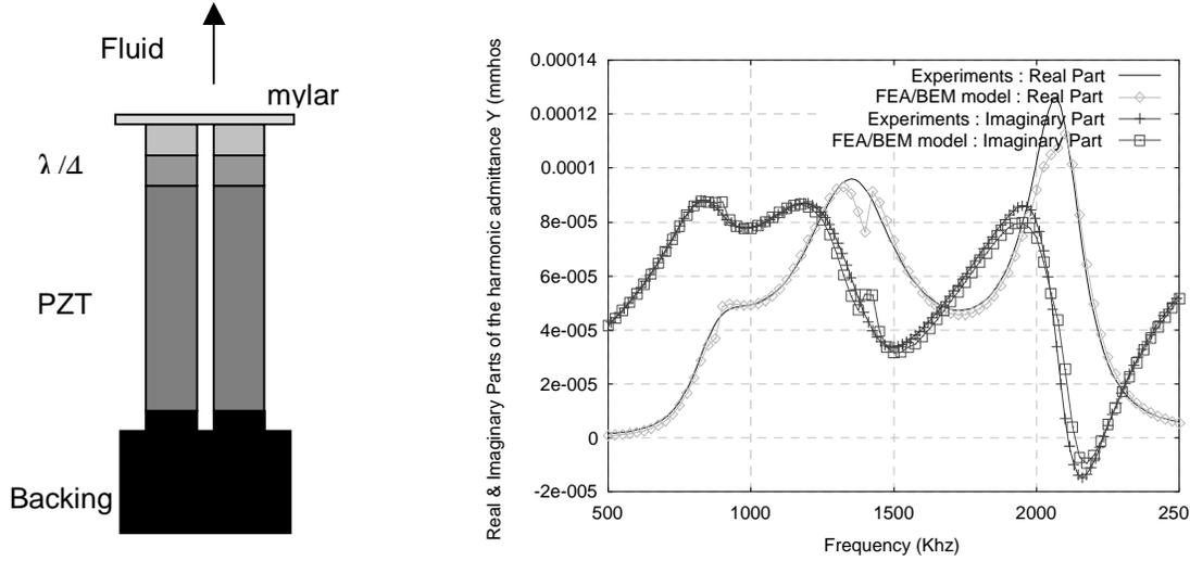
Fig.5 Typical structure of a standard imaging probe, predictions of its response when radiating in water
