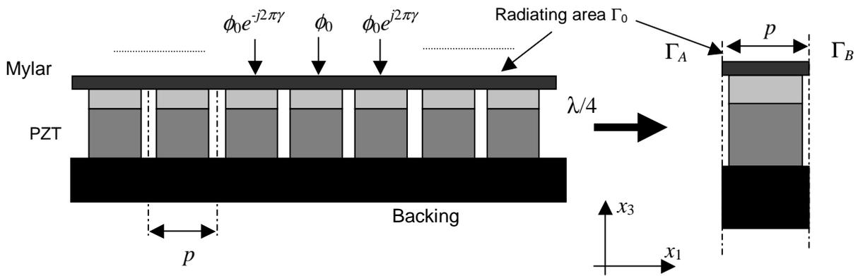
Fig.2 Scheme of a periodic structure represented by only one period
