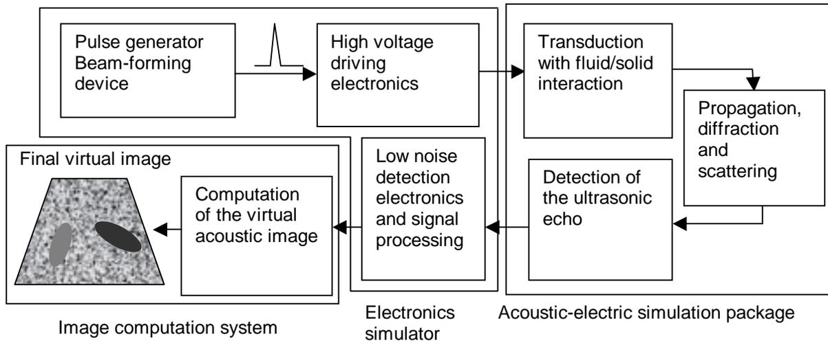
Fig. 1 Scheme of the principle of an ultrasonics virtual laboratory
