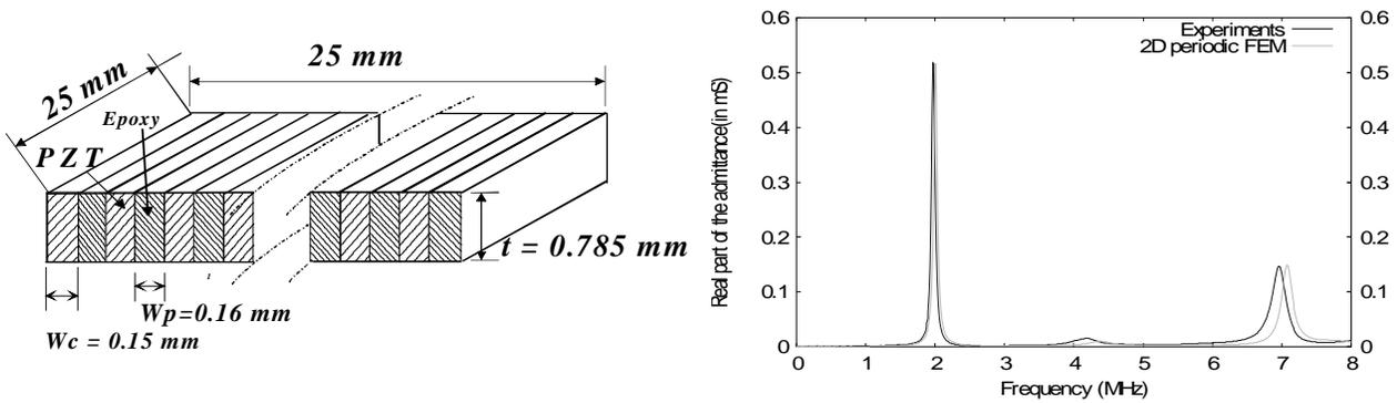
Fig.3 Prediction and measurement of the auto-admittance of the described 2-2 piezocomposite
