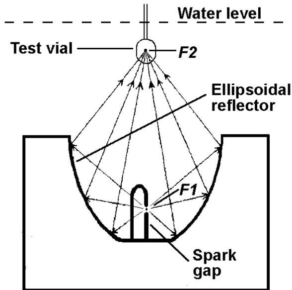
**Fig. 1. Schematic diagram of the electrohydraulic shock wave generator.**
