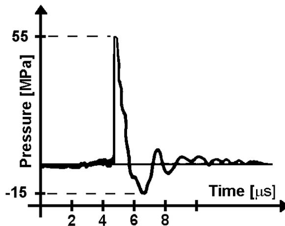
**Fig. 2. Pressure profile obtained with a PVDF needle hydrophone positioned at the  $F2$  focus of the electrohydraulic shock wave generator.**
