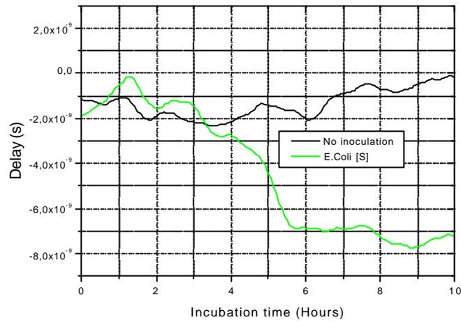
Figure 3. Time of flight delay (s) as a function of the incubation time. The green line represents the delay of the inoculated sample measured with the transducers at opposite sides of the bottle ("S" configuration). The black line is the delay time registered at a reference bottle.
