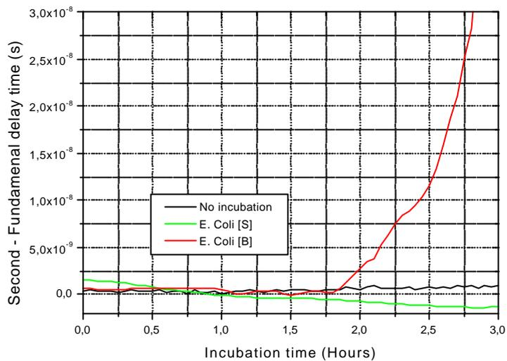
Figure 7. Difference between Second harmonic and fundamental time of flight delay as a function of the incubation time. The green and red lines belong to the inoculated samples measured with “S” and “B” configurations, respectively. The black line is the second harmonic amplitude registered at a reference bottle.
