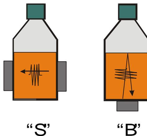
Figure 1. “S” configuration: two transducer placed in the opposite sides of the culture bottle. “B” configuration: One transducer array placed at the bottom of the culture bottle, with the ultrasonic tone-burst being reflected at the liquid-gas interface.
