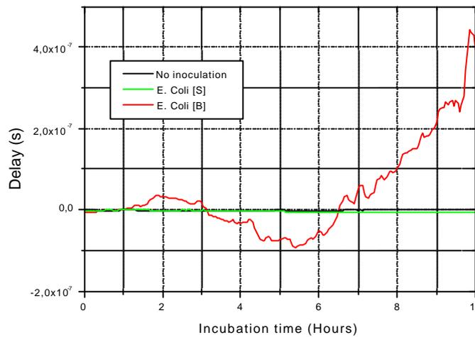
Figure 4. Time of flight delay (s) as a function of the incubation time. The green and red lines represent the delay of the inoculated samples measured with "S" and "B" configurations, respectively. The black line is the delay time registered at a reference bottle.
