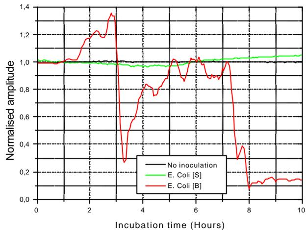
Figure 5. Normalised amplitude as a function of the incubation time. The green and red lines represent the amplitude of the inoculated samples measured with “S” and “B” configurations, respectively. The black line is the amplitude registered at a reference bottle.
