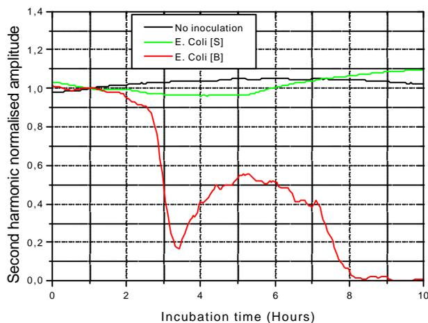
Figure 6. Second harmonic amplitude as a function of the incubation time. The green and red lines represent the second harmonic amplitude of the inoculated samples measured with “S” and “B” configurations, respectively. The black line is the second harmonic amplitude registered at a reference bottle.
