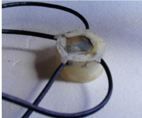
Figure 2. Photograph of the 2-4MHz transducer array.
