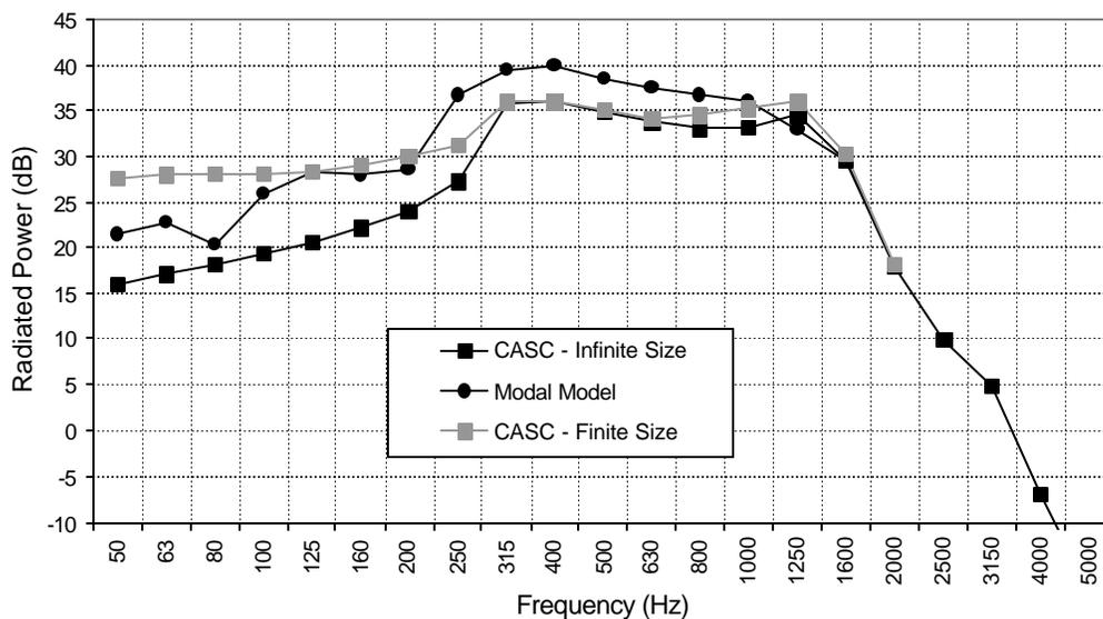
Figure 4: Sound radiated power for the double glazing.
