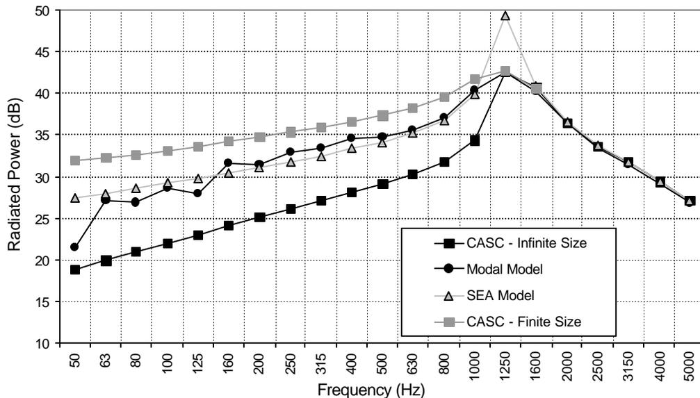
Figure 3: Sound radiated power for the single glazing.
