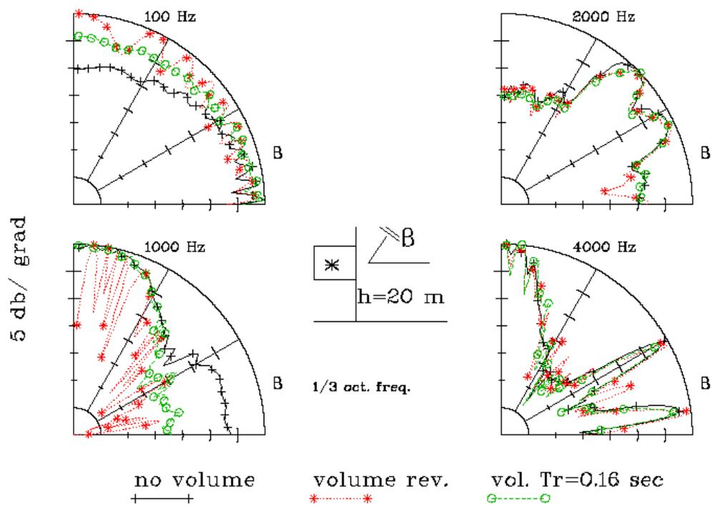
Figure 6. Influence of angle of incidence of incoming wave on transmitted SPL.
