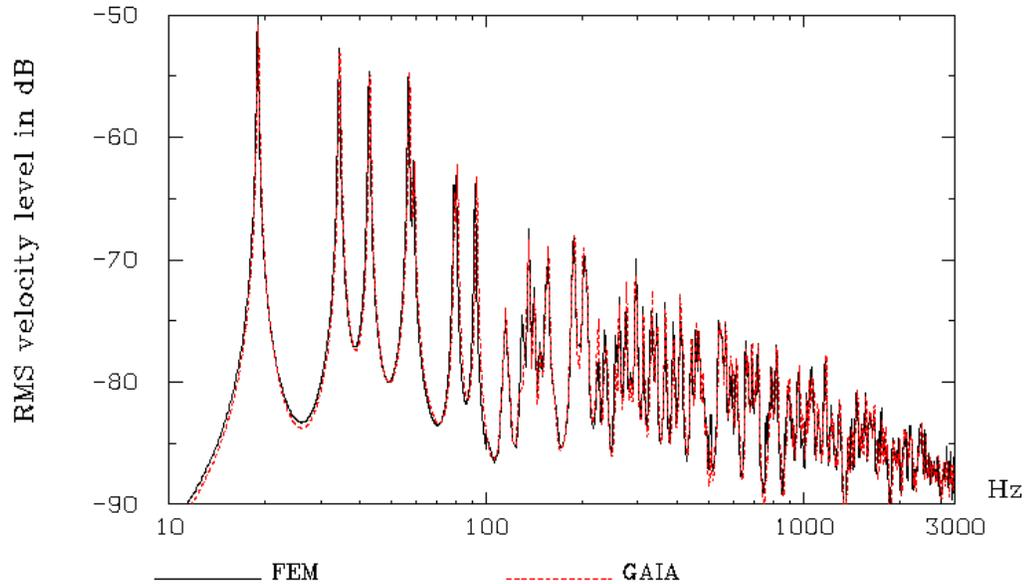
Figure 1. Plaster 3x2.5 M2, 5 cm-thick clamped plate. Unit force at (0.9,0.75).
