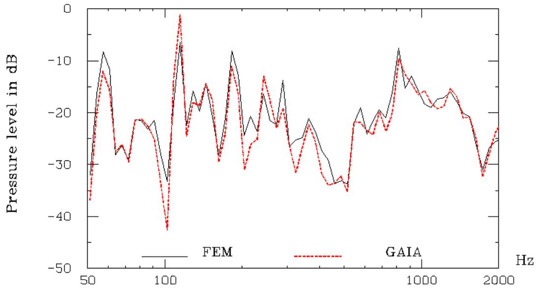
Figure 4. Transmitted SPL through a 5 cm clamped plaster wall between 2 volumes.
