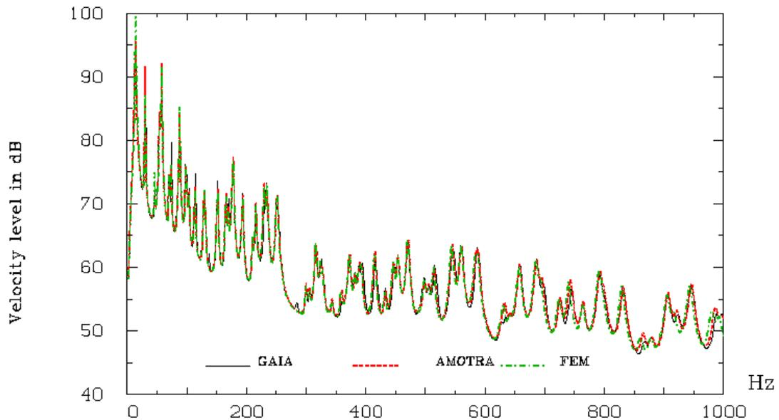
Figure 2. Velocity level of a SCSC 5-cm plaster plate excited by a (30,30) deg plane wave.
