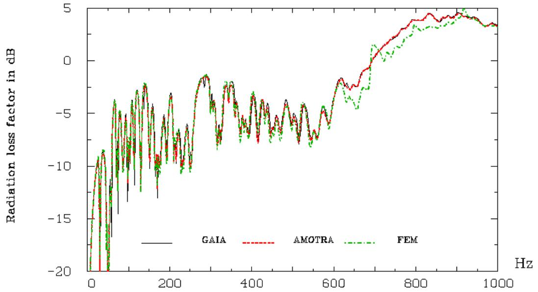
Figure 3. Radiation loss factor. SCSC 5 cm-thick plaster plate.
