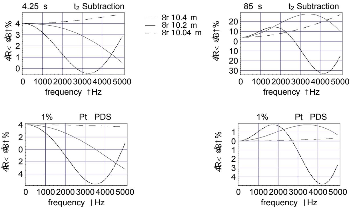
Figure 2: The bias error  $\Delta|R(\omega)|$  of both extraction techniques.
