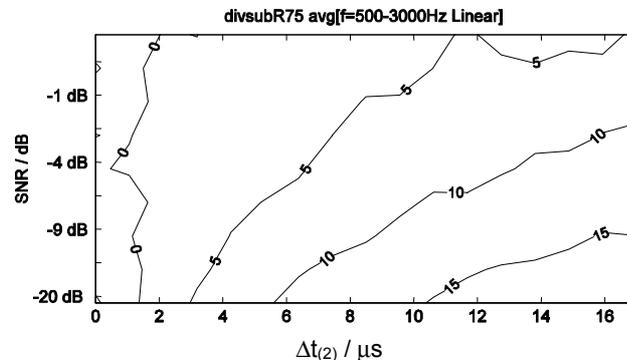
Figure 4: The calculated logarithmic ratio of the single error number occurring by the application of the 'Subtraction'-technique related that of the 'PDS'-technique
