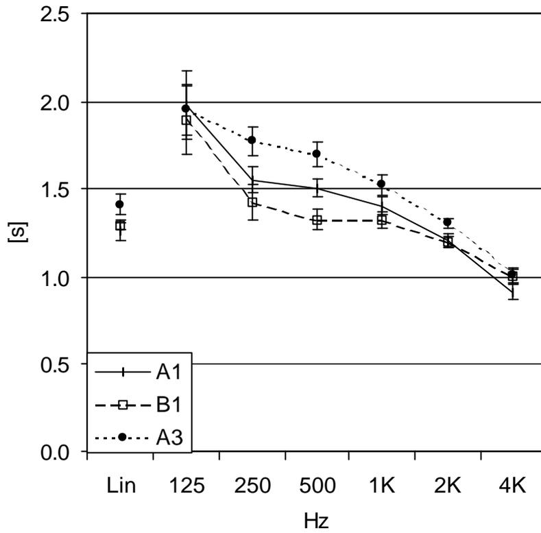
Fig. 4 – The parameter RT20 measured in the stalls of the theatre for the three sound source positions A1, A3 and B1.
