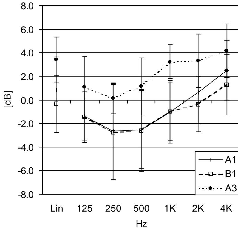
Fig. 5 – The course of the clarity C80 in the stalls for the different positions of sound source. The error bars refer to one standard deviation.
