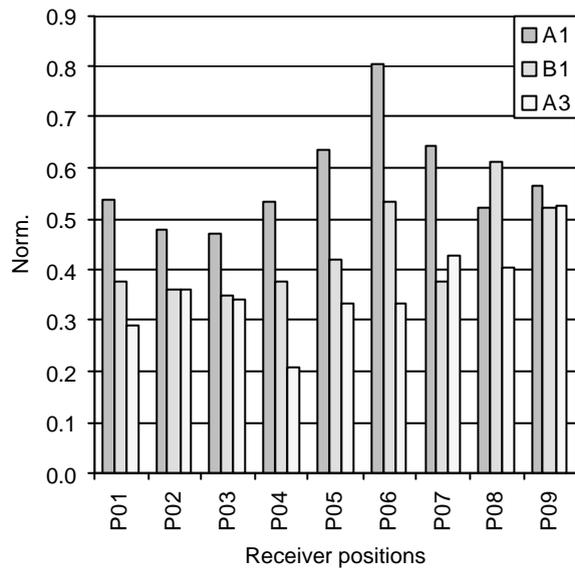
Fig. 7 – The values of lateral fraction LF in the stalls.
