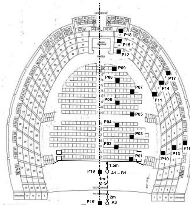
Fig. 3 – The plan of the sound sources and of the receivers employed for the measurements in the theatre.
