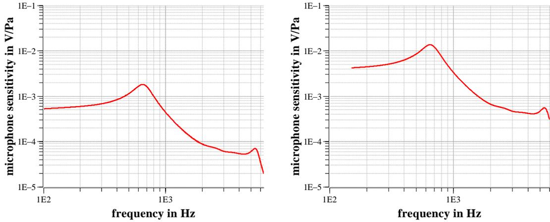
**Figure 2:** Numerical simulations: predicted best performance of the implantable microphone. **Left:** PZT hollow cylinder. **Right:** PZT coated bending plate.
