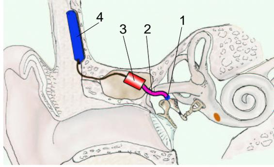
**Figure 1:** Principal design of the hydroacoustic microphone: Ossicle vibrations are picked up by a diaphragm (1) coupled to a fluid-filled tube (2) with subsequent transduction of the fluid sound field into electrical signals by a piezoelectric sensor device (3) placed in the mastoid. Also shown is the CI processor unit (4).
