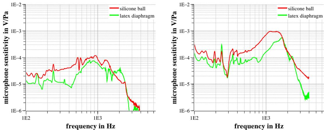
**Figure 3:** Temporal bone experiment: Sensitivity of implantable microphone prototypes. Note that the piezoelectric elements were of non-optimal dimensions. **Left:** PZT hollow cylinder. **Right:** PZT coated bending plate.
