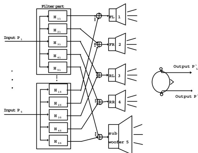
Fig. 3 5-channel sound reproduction system in the automotive space
