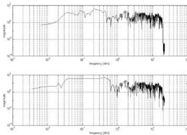
Fig. 5 Frequency response of before-equalization (up) and after-equalization (down)
