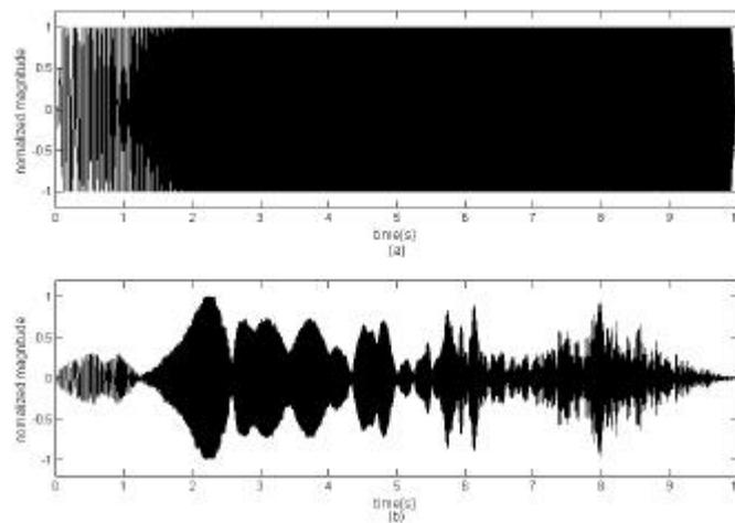
Fig. 2 (a) input log sweep signal, (b) one of the recorded binaural signals
