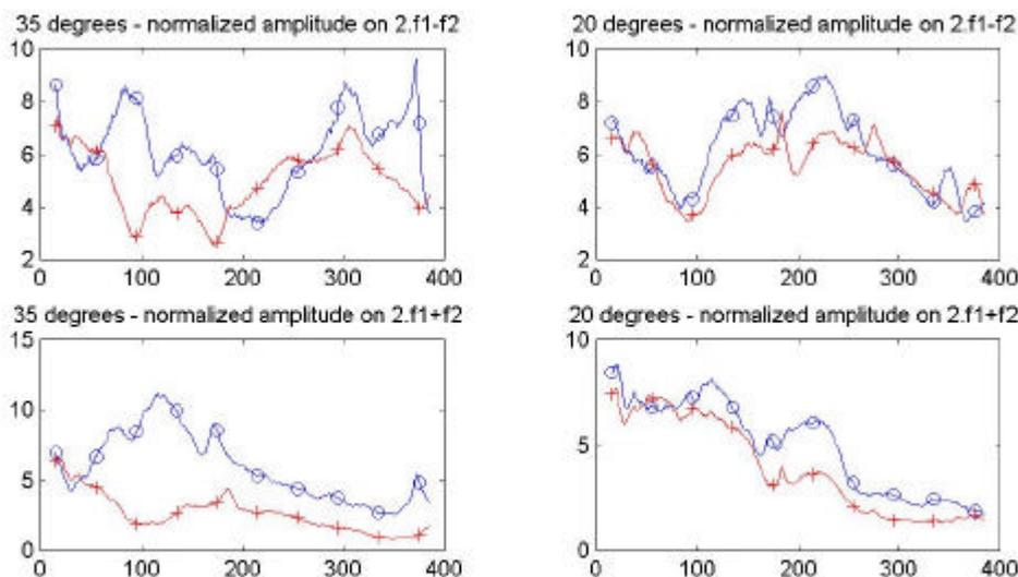
Figure 10: Global results of the normalized amplitude for the two angles and the two duration time of annealing (+) for  $t_1=7$  mn and (o) for  $t_2=17$ mn
