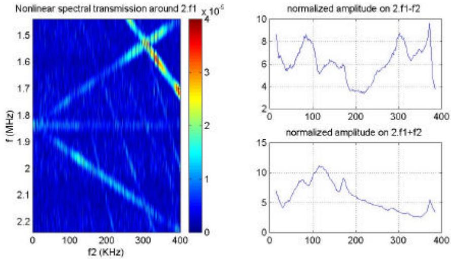
Figure 7: Results for plate 2 ( $t_1=17$  mn) spectral results for  $\theta=35$   $f_1=0.92$ MHz
