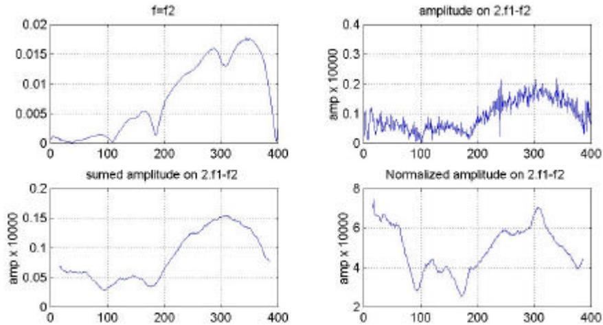
Figure 5: Amplitude measurement on oblique lines of the spectral results, (Plate 1:  $t_1=7mn$ ,  $f_1=1.19MHz$ ,  $\theta=35degrees$ ).
