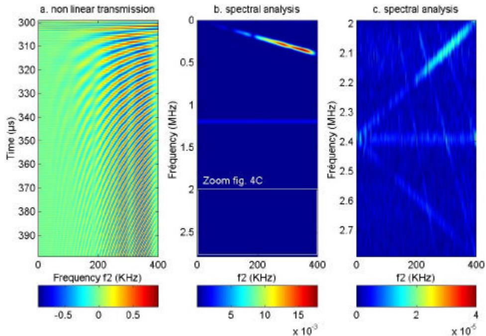
Figure 4: Plate 1 ( $t_1=7\text{mn}$ ,  $f_1=1.19\text{MHz}$ ), temporal and spectral results, transmission for  $\theta=35\text{degrees}$
