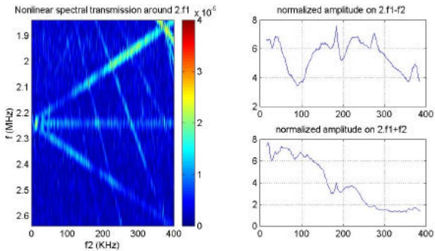
Figure 8: Results for plate 1 ( $t_1=7$  mn) spectral results for  $\theta=20$   $f_1=1.12$ MHz
