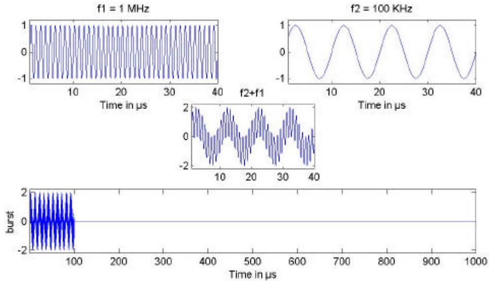
Figure 3: Building of the emitting signal
