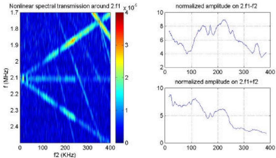
Figure 9: Results for plate 2 ( $t_1=17$  mn) spectral results for  $\theta=20$   $f_1=1.05$ MHz
