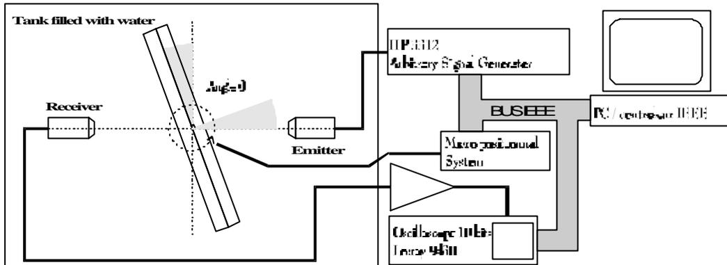
Figure 1: Experimental setup: bistatic method.
