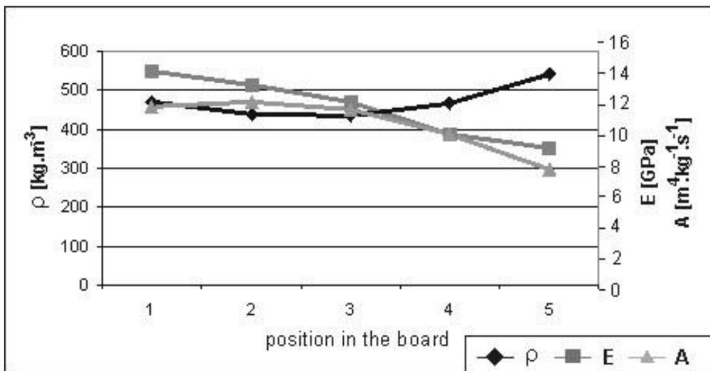
Fig. 3 Density, E-modulus and acoustical constant along the plate R13a
