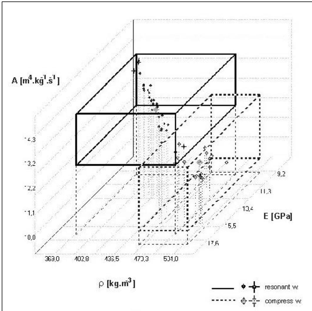
Fig. 4. Density  $\rho$ ,  $E$ -modulus and  $A$ -constant of high-quality resonant spruce wood (mjstr) and set of compression spruce wood (reak12) at the reference moisture content 12 %
