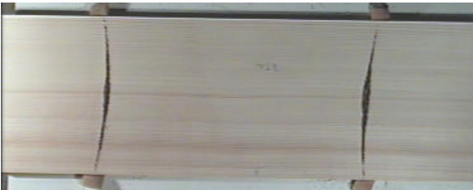
Fig. 1 The Chladni pattern (2,0) of the tested plate R5a on  $f = 154$  Hz
