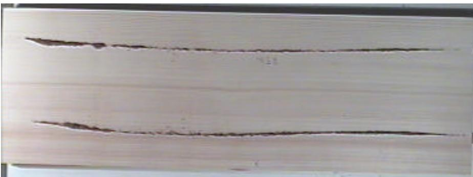
Fig. 2 The Chladni pattern (0,2) of the tested plate R5a on  $f = 348$  Hz
