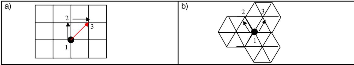
Figure 4 Evolution of the wave front in a square (a) and an hexagonal (b) mesh.
