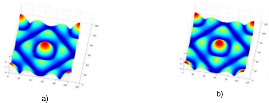
Figure 6(a) and 6(b): modal constraints obtained for 551 Hz (order 1) and 547 Hz (order 2)
