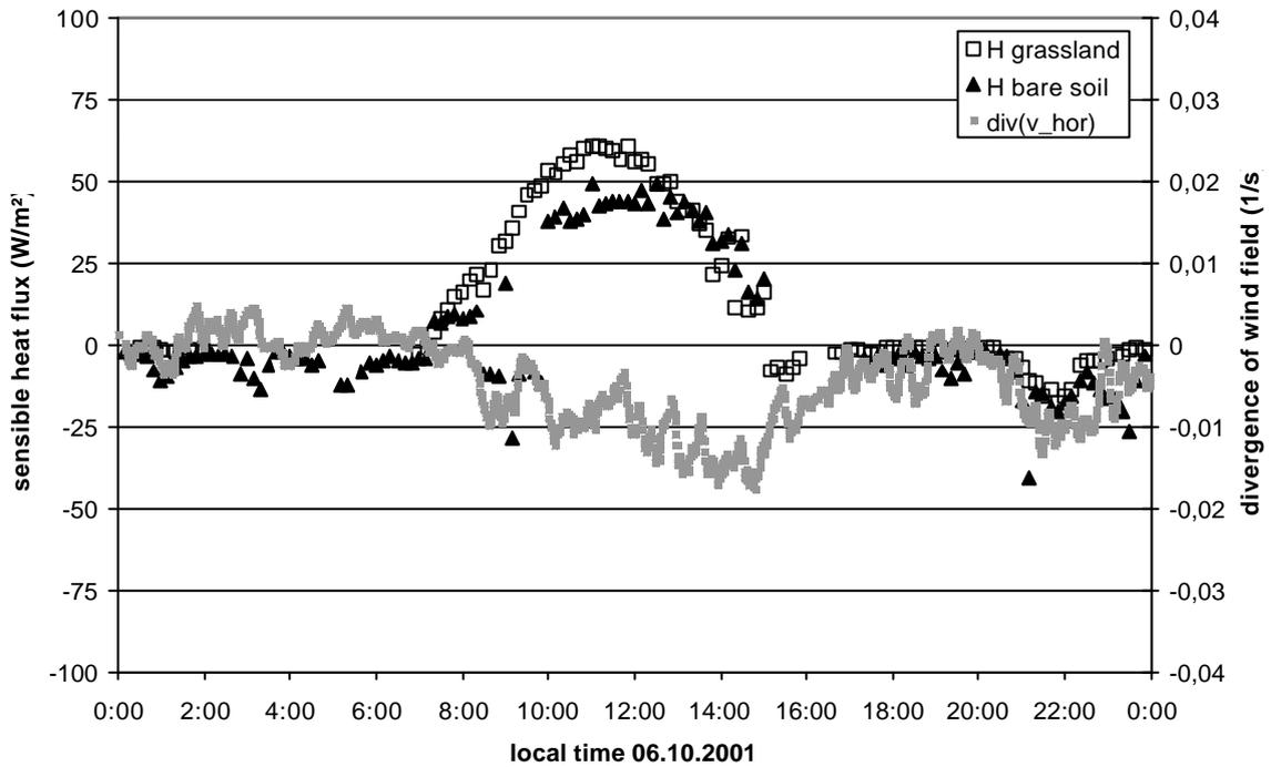
**Fig. 3:** Diurnal course of the vertical sensible heat fluxes measured with the scintillometer SC1 over grassland and SC2 over bare soil (for positions see Fig. 1) in comparison to the tomographically observed divergence in the horizontal wind field.
