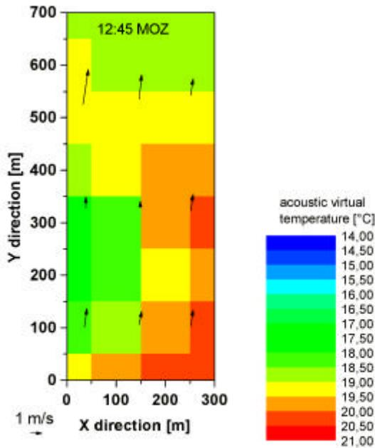
**Fig. 4:** Tomogram of the acoustic virtual temperature (32 cells) and wind speed (arrows in 9 cells) on the 6 October 2001 at 12:45 MOZ (local time).
