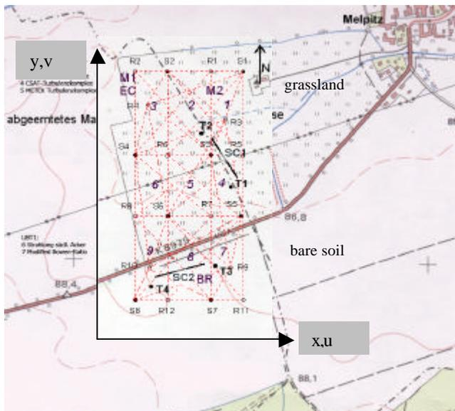
**Fig. 1:** Layout of the area under investigation ( $300 \times 700 \text{ m}^2$ ) at the research station Melpitz. The northern part was grassland and southerly of the road was bare soil (acre). The dotted lines represent the acoustic rays between source and receiver of the tomographic array and the numbers (1...9) are the wind cells.
