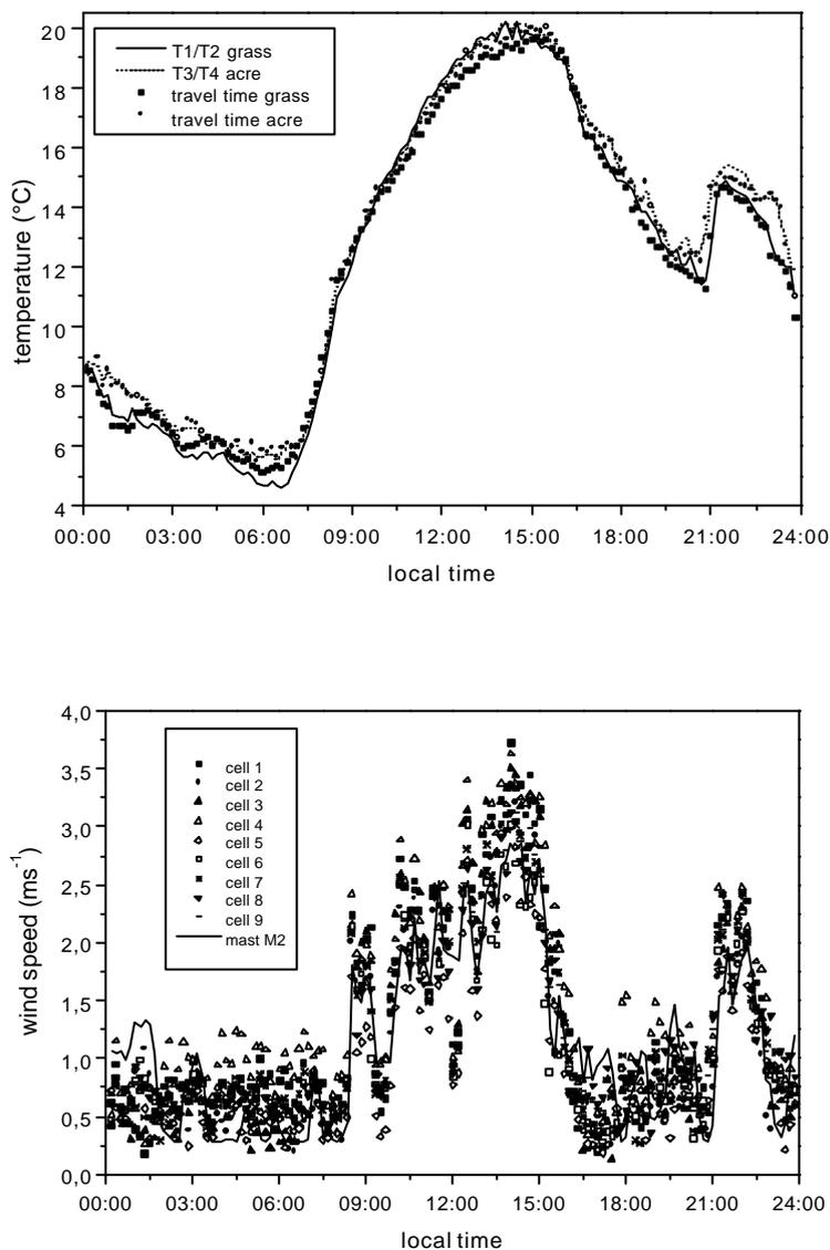
**Fig. 2 :** Experiment STINHO-1: Comparison of air temperature and wind measurements 06.10.2001. Diurnal course of the
