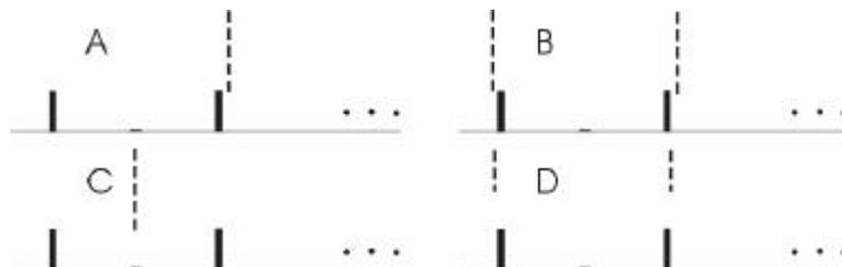
Figure 2. Overview of the double noise barrier configurations under investigation
