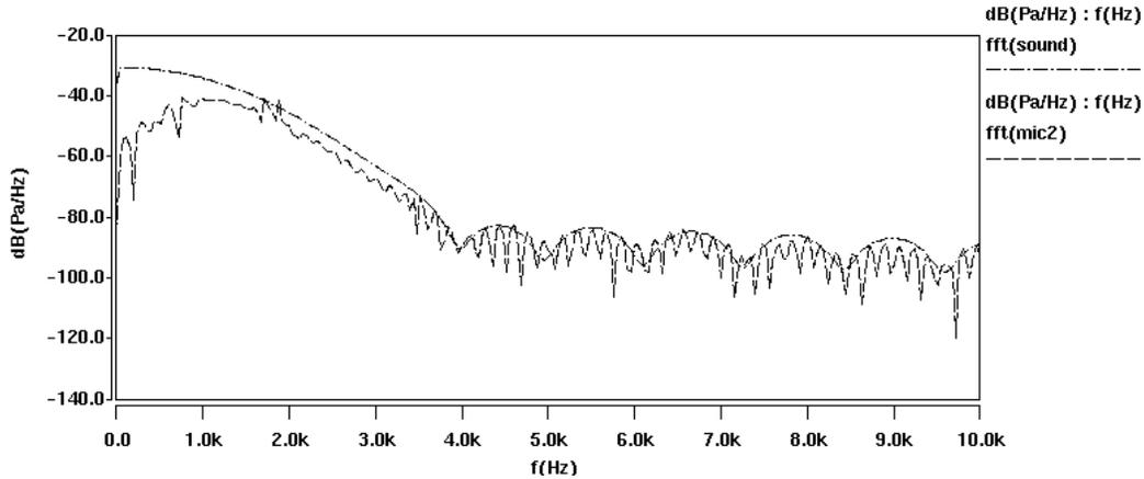
Figure 3: Power spectral density of Gaussian shaped input impulse and the sound pressure at the exit of the pipe.
