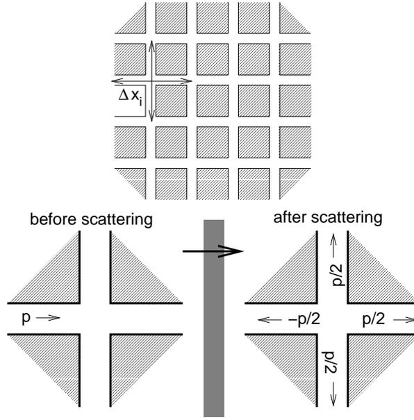
Figure 1: The acoustic medium is replaced by a network of pipes, in which pressure waves travel. The junctions are called nodes, the vectors  $\Delta \vec{x}_i$  point from one node to the nearest neighbors. The scattering process is depicted in the lower part of the figure.
