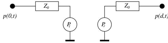
Figure 2: Equivalent circuit model for the lossless transmission line, which corresponds to the pipes in the TLM mesh.
