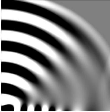
Figure 4: Snapshot of the pressure field over a compliant wall. The wall is at the bottom boundary, at the top and right absorbing boundary conditions were applied while the left boundary condition was set to ideal reflection. Grey means average pressure while white and black corresponds to areas of higher/lower pressure, respectively. The black and white patterns along the bottom boundary belong to surface waves, which decay exponentially away from the surface.
