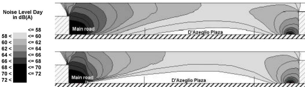
Figure 4: Acoustic simulations in the actual state (left) and in the project (right) for the square.
