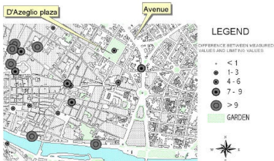
Figure 2: Difference between measured sound pressure level in the daytime and acoustical class limits.
