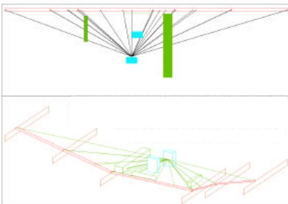
This latter method has the advantage of producing a steady change in results for any minor displacement of receptor position. Within any sub-segment it creates, the barrier influence also changes reasonably steadily so that assuming one representative position still leads to high accuracy results.
