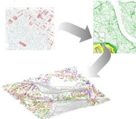
During recent years Laser Scan Data collected from aircraft have become available. This can be used to automatically generate a 3-d model though it cannot recognize whether an object is "non stationary".
