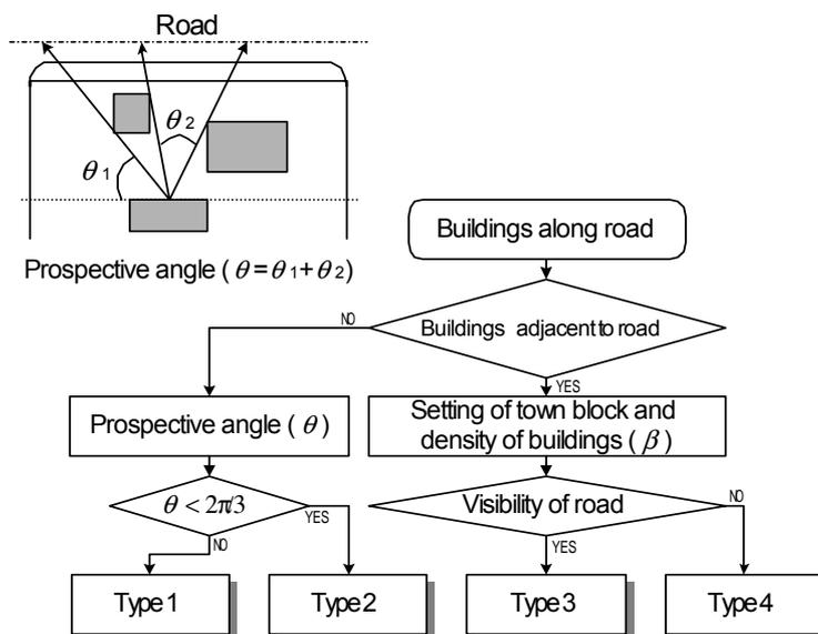
Fig. 1. Outline of predicting method of road traffic noise proposed in the Manual [2].
