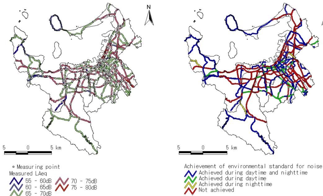
Fig.2. Measured noise levels ( $L_{Aeq}$ ) at roadside.
