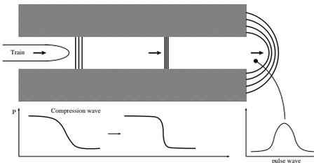
Figure 1: The low frequency noise from a tunnel
