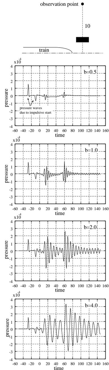
Figure 8: Pressure histories observed away from the structure in the lateral direction
