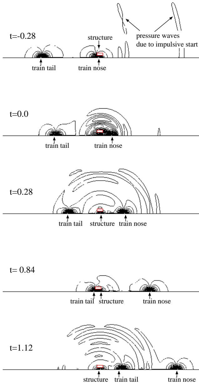
Figure 7: Pressure contour plots when the train passes through the structure ( $b=1$ )
