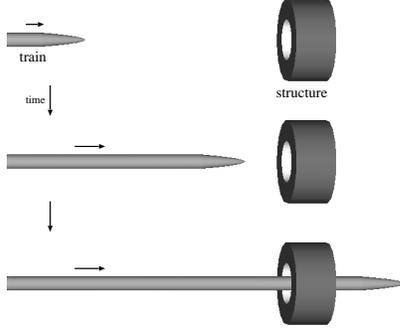
Figure 3: An axisymmetric flow field model where a train passes through a structure
