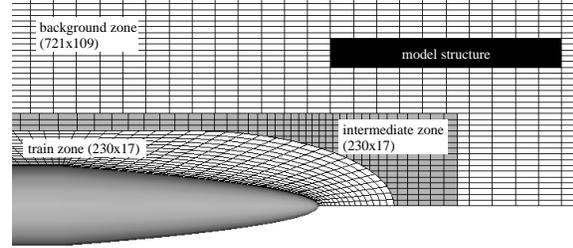
Figure 6: The zone geometry and the grid distributions
