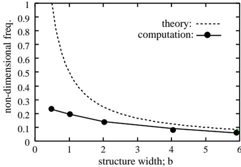
Figure 9: The non-dimensional frequency of the pressure wave compared with the resonance frequency.
