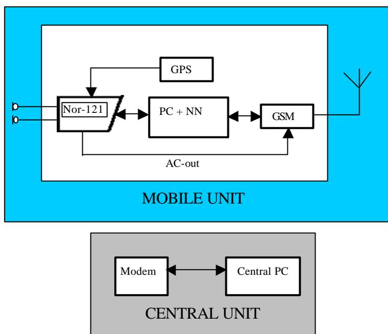
Figure 2 Complete monitoring system.
