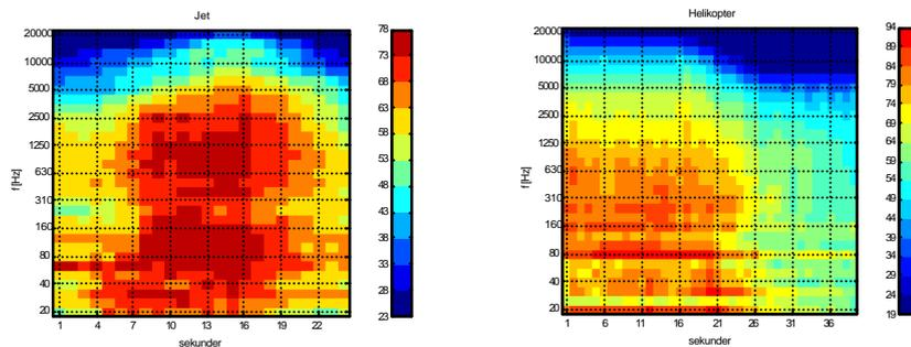
Figure 1B Spectra as a function of time for a jetplane (left) and a helicopter (right). Resolution along the y-axis is 1/3 octave band, with the center frequency as the label. The level in dB is given by the colour.
