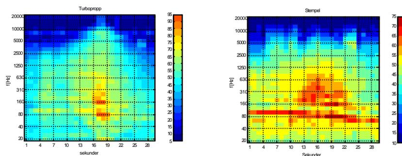
Figure 1A Spectra as a function of time for a turbo prop (left), and a piston engine (right). Resolution along the y-axis is 1/3 octave band, with the center frequency as the label. The level in dB is given by the colour.
