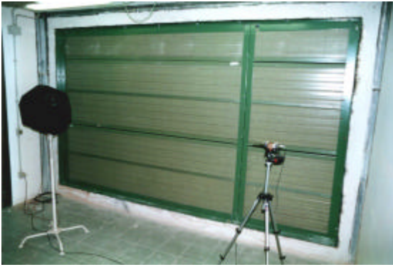
Fig. 2: sample I of the noise barrier (only bored metal panels)
