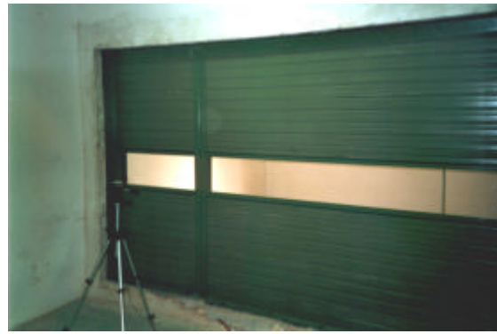
Fig. 3: sample II of the noise barrier (PMMA and bored metal panels)
