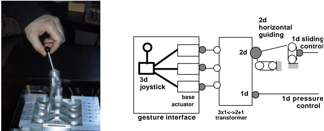
**Figure 2. The 3d bowing force feedback joystick and its coupling to the bow simulation.**
