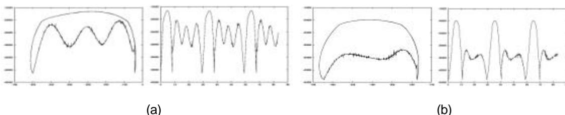
**Figure 5. The bowing force observed (coil current) for two different values of the damping coefficient in the string: low damping (a) and high damping (b). The left diagrams (force versus string displacement) area is the energy supplied to the string at each cycle.**
