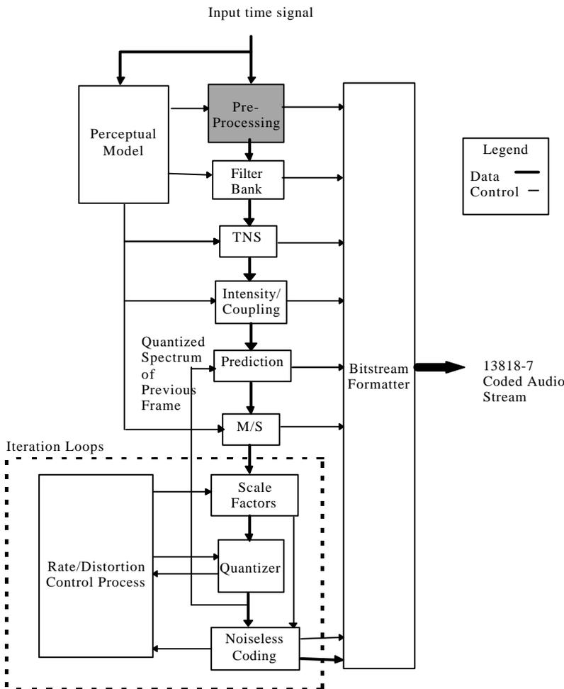
Fig 3: Block diagram of MPEG-2 Advanced Audio Coding
