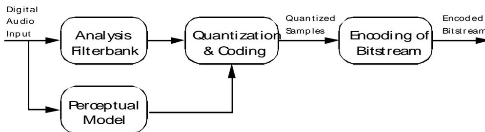
Figure 1: Block diagram of a perceptual encoding/decoding system.
