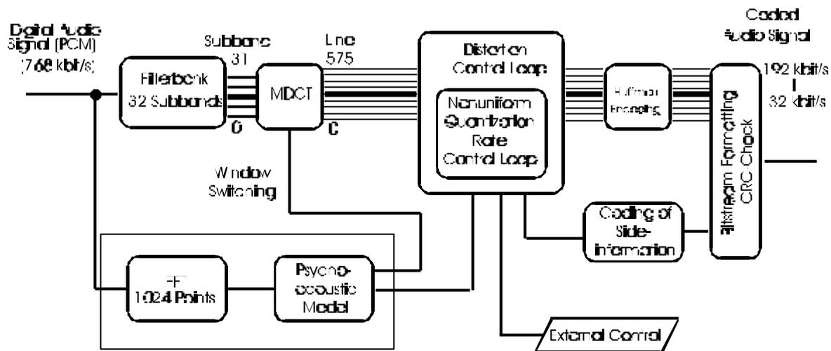
Fig. 2: Block diagram of MPEG Layer-3 (MP3) encoding
