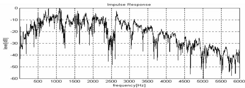
Fig. . Impulse response of the top plate only
