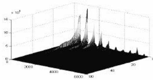
Fig. . 3D-spectrogram of the plucked string
