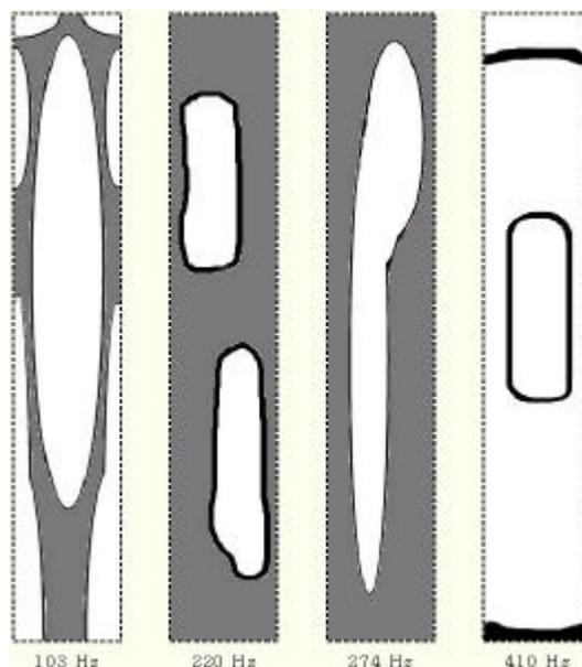
Fig. . Chladni patterns of the complete body
