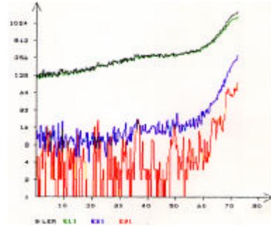
Every obstacle (on optical disc here) will improve error rate. On the right example, error correction processing can't compensate such an increasing level at the end of the disc.
