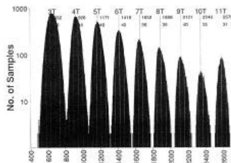
Exemple of Jitter histogram corresponding to each pit lengths of a CD-R. Some confusion are possibles in recognising 3T/4T to 5T/6T.
