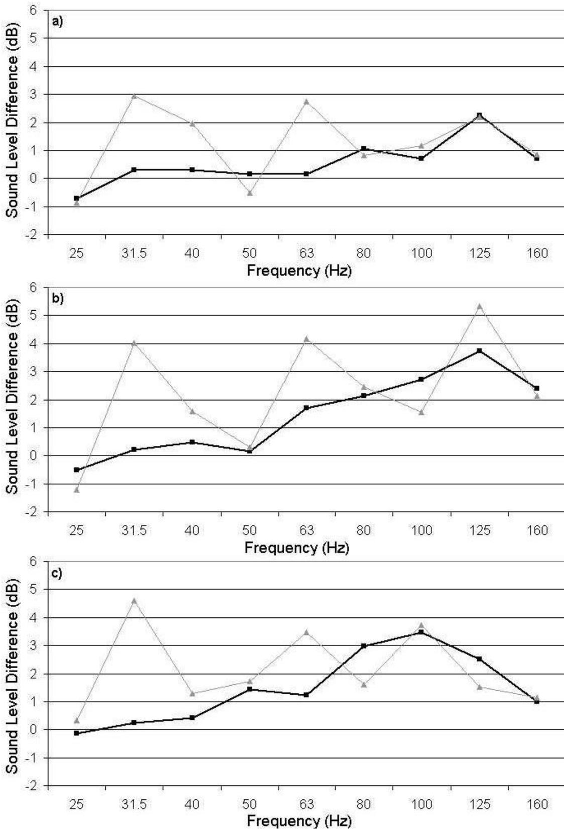
Figure 6 - Level difference (—■—) between measured values and (---▲---) between predicted values. Results shown in one-third octave bands. a) Central floor position, b) centre wall position, and c) corner position.
