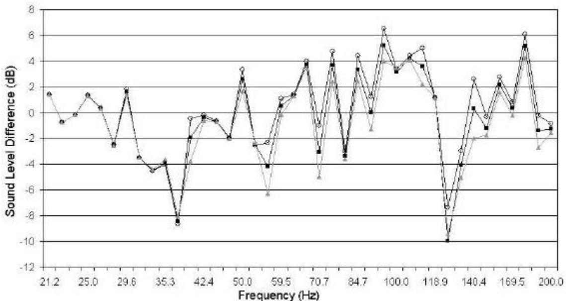
Figure 2 - Level differences between measurement and prediction of Chair model at centre wall position. (—○—)  $a=30\%$ , (—■—)  $a=50\%$ , and (—▲—)  $a=70\%$ .
