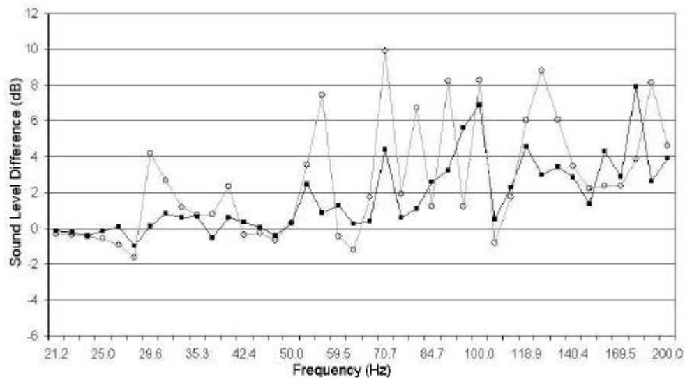
Figure 4 - Results for the armchair in the centre wall position: comparison between (—■—) measured and (---○---) predicted level differences in 1/12<sup>th</sup> octave bands.
