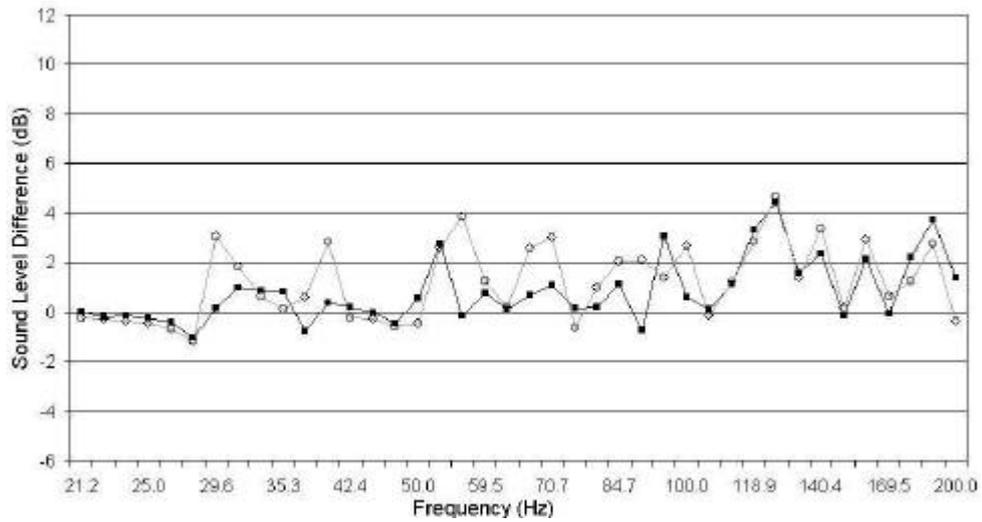
Figure 3 - Results for the armchair in the centre of the room floor: comparison between (—■—) measured and (---○---) predicted level differences in 1/12<sup>th</sup> octave bands.
