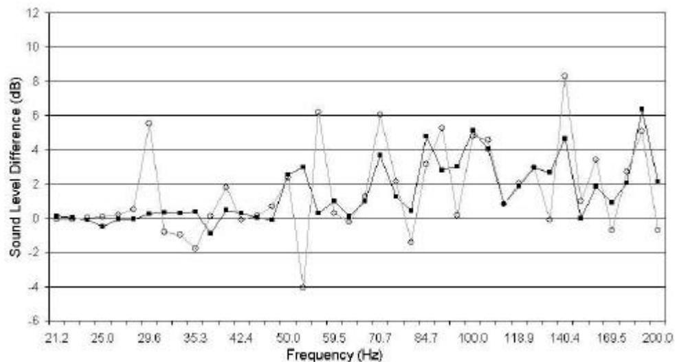
Figure 5 - Results for the armchair in the corner position: comparison between (—■—) measured and (---○---) predicted level differences in 1/12<sup>th</sup> octave bands.
