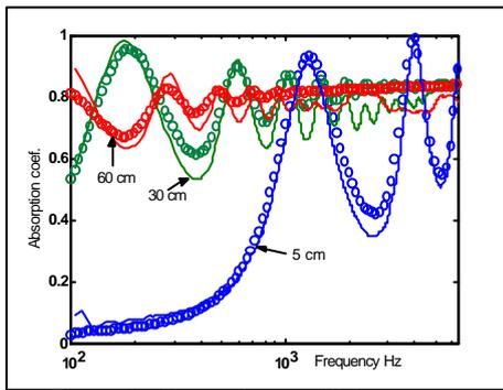
Figure 2. Absorption coefficient versus frequency for three layer thickness
