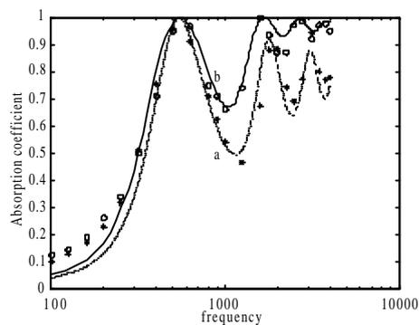
Figure 3. Calculated (continuous lines) and measured absorption of a cylinder and a wedge of granular material with identical volume.
