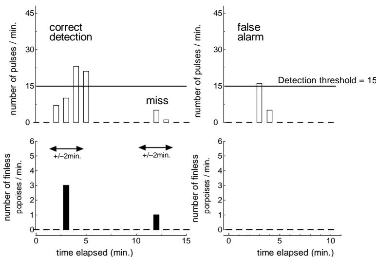
FIG.3 Schematic of correct detection, miss and false alarm of the acoustical observation system. A time window centered at the visual detection was depicted as two arrows. The acoustical correct detection of the animals was defined that the number of the observed pulses in a minute within the time window was more than 15. The acoustical miss was defined as the less number of pulses in a minute within the time window.
