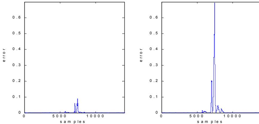
Figure 2. Two error functions, obtained comparing signatures from same and distinct equipment respectively.
