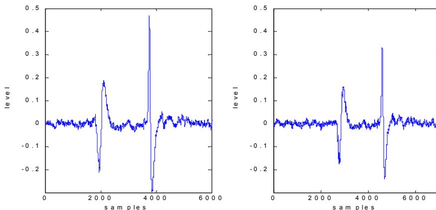
Figure 3. Differences between same erase head marks obtained without and with azimuth deviation respectively.
