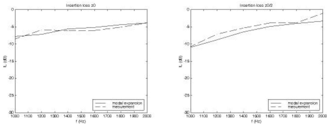
Figure 4: Comparison of predicted and measured values of the Insertion Loss
