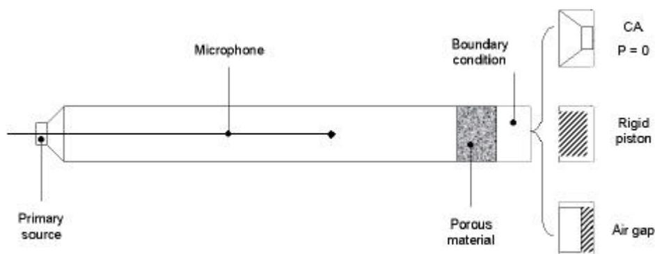
Figure 5 : Experimental set-up, the standing wave tube.
