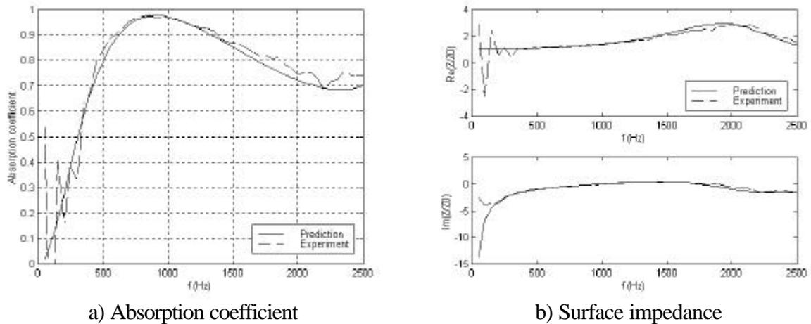
Figure 6 : Comparison between prediction and measurement for a 25 mm felt :
