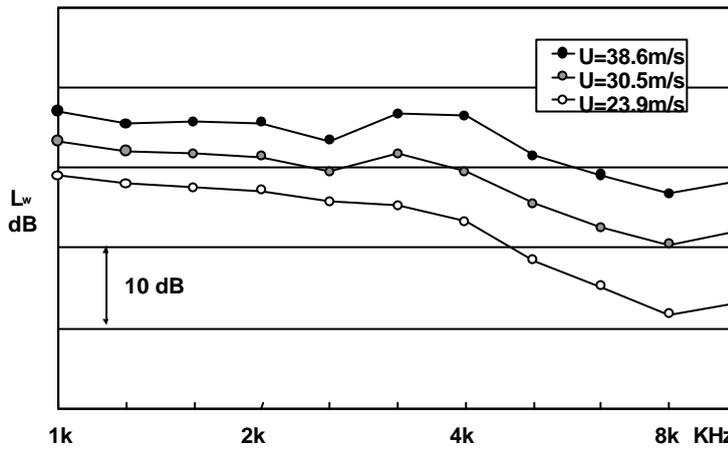
Figure 2. Effect of flow velocity on sound power radiated by panel 2.
