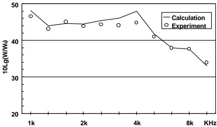
Figure 7. Comparison of predicted and measured sound power radiated by panel 3.
