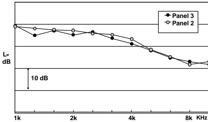
Figure 1. Sound power radiated by different panels excited by pressure fluctuations from 3 mm-high steps at  $U=23.9$  m/s.
