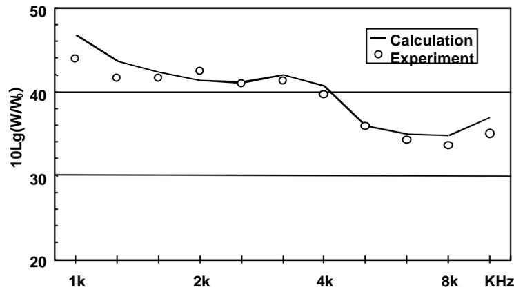
Figure 6. Comparison of predicted and measured sound power radiated by panel 1.
