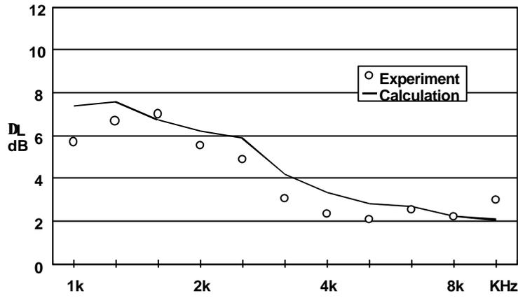
Figure 5. Comparison of predicted and experimental increases in sound-radiation for panel 3.
