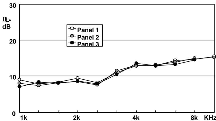
Figure 3. Variation of sound power radiated by different panels excited by the pressure-fluctuation field from steps when flow velocity is increased.
