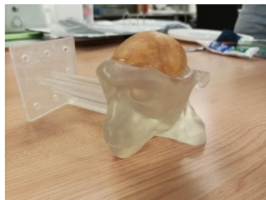
Figure 1 - Head mimicking of a non-human primate by assembling an ex-vivo skull and a 3D-printed head.
