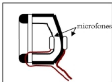
Figure 1 – Schematic representation of the microphones position inside and outside the HPD.
