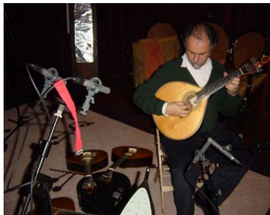
Figure 1 – Picture of the recording setup, showing the A-B microphone pair (on the left side of the picture) and the sound level meter location.
