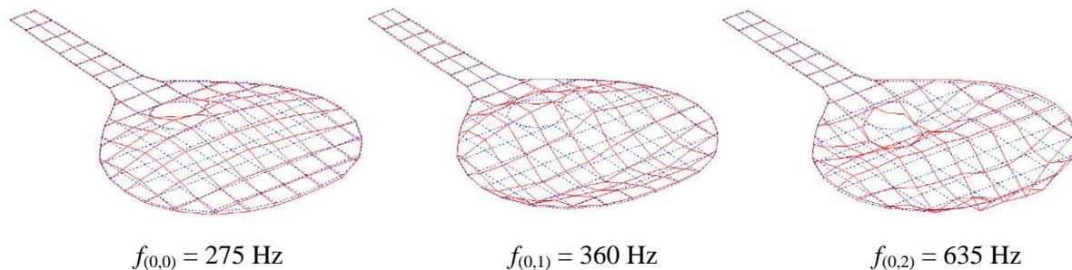
Figure 6 – Modeshapes of three resonances of the soundboard of guitar D.
