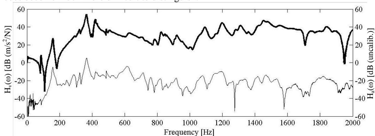
Figure 3 – Example of an accelerance (heavy line) and vibroacoustic (thin line) frequency response function of guitar E.
