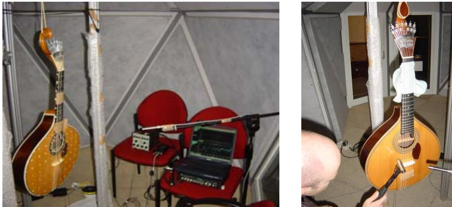
Figure 2 – Experimental setup showing the impact test positions and the location of the microphone for the vibroacoustic transfer functions measurements.
