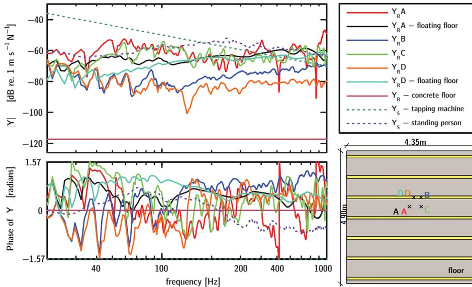
Figure 9 – Floor and source mobilities. Note the dependence on the source position on the timber joist floor (after [10])
