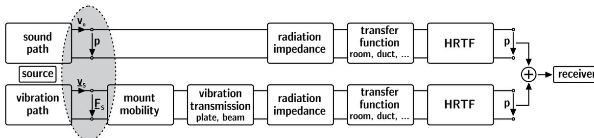
Figure 5 – Detailed block diagram of binaural transfer path synthesis (after [1])
