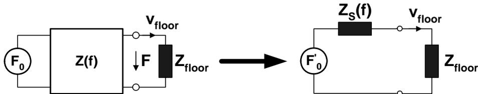
Figure 7 – Definition of a real vibration source with blocked force  $F_0$  and inner impedance  $Z_s$ .
