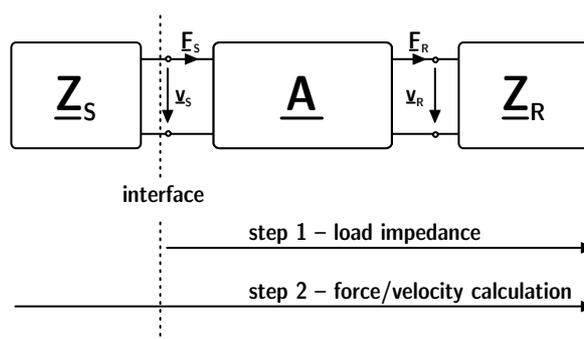
Figure 6 – Two-port as a central coupling element of TPA (after [1]).
