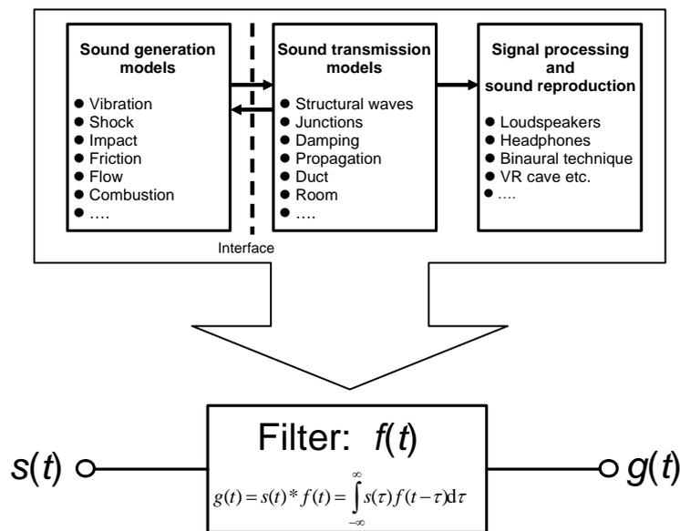
Figure 2 – Projection of the vibroacoustic signal path into a signal processing model ([1]).
