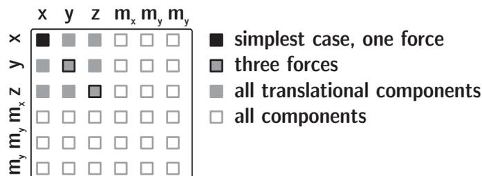
Figure 4 – Impedance or mobility matrix representation showing the six degrees of freedom and the interaction between them.
