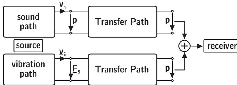
Figure 1 – Simplified block diagram of transfer path synthesis (after [1])
