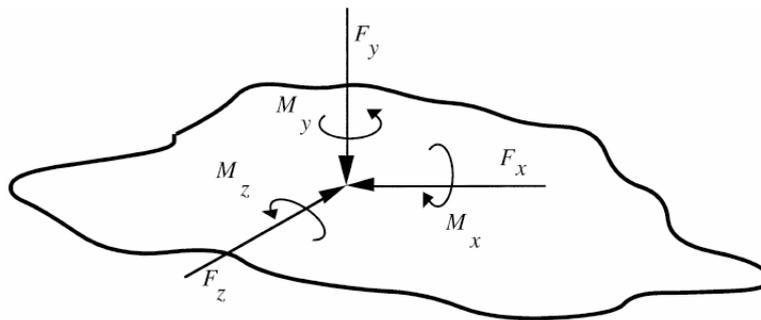
Figure 3 – Point contact of a source with complex description of the force transmission, three orthogonal forces and three moments (after [2]).
