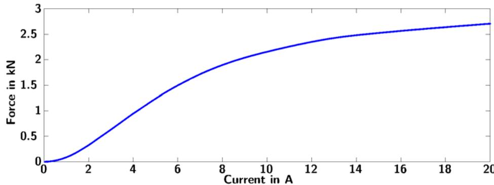
Figure 2: Relation between phase current and radial force
