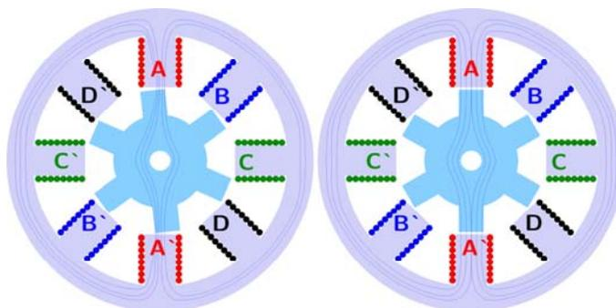
Figure 1: Schematic representation of a switched reluctance machine (SRM)
