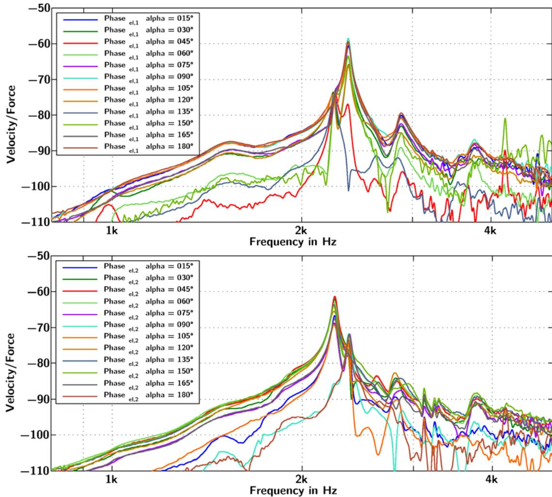
Figure 6: Measured transfer function for the first electrical phase (top) and for the second electrical phase (bottom)
