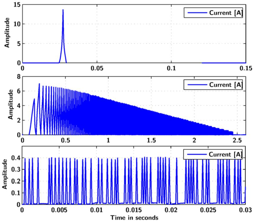
Figure 4: Broad band current signals used for the measurement. From top to bottom: pulse, sweep, pseudo-random noise (only a short window of the pseudo-random noise signal is plotted).
