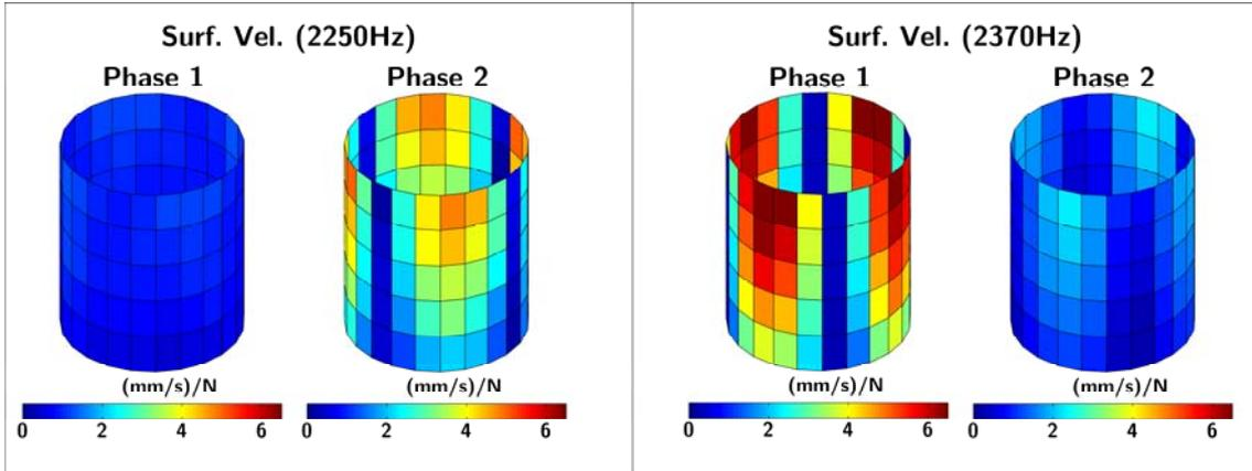
Figure 7: Plot of the measured surface velocity on a cylinder representing the stator. Of the four measurements (applying the current signal to one of the four electrical phases), only the results for two of them are plotted. On the left-hand side plot are for a frequency of 2250 Hz, on the right hand side for 2370 Hz.
