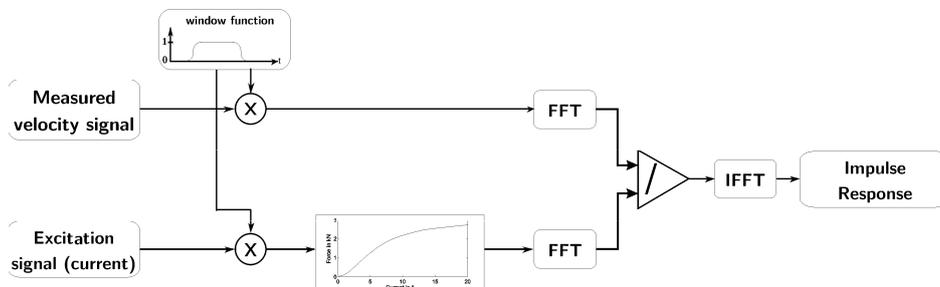
Figure 3: Diagram of the impulse response (transfer function) calculation
