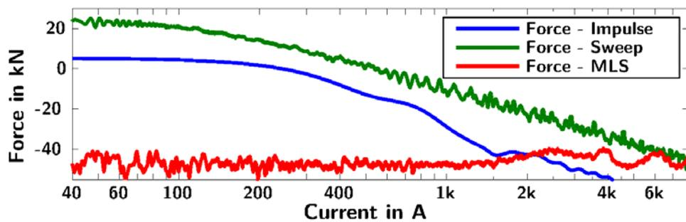
Figure 5: Spectrum of the three broad band force excitation signals
