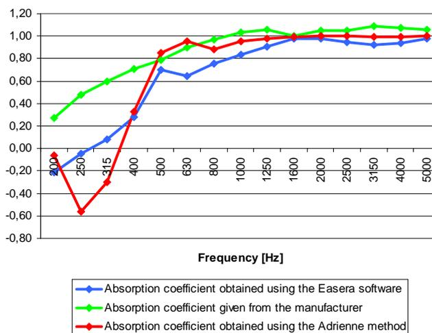
Figure 7: Comparison of absorption coefficient data gained using the Easera software, the Adrienne method and the data given by the manufacturer of the tested device.
