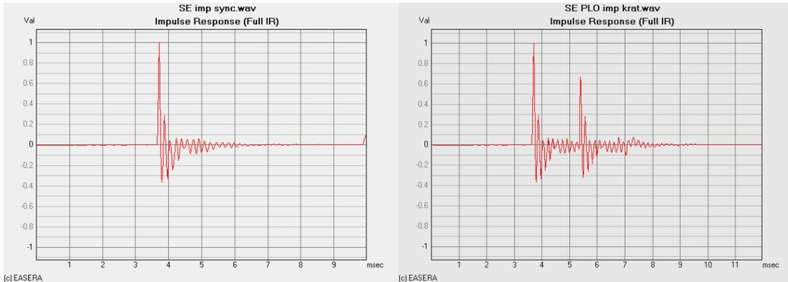
Figure 4: Impulse responses in the measurement position: left – free field, right – hard surface.
