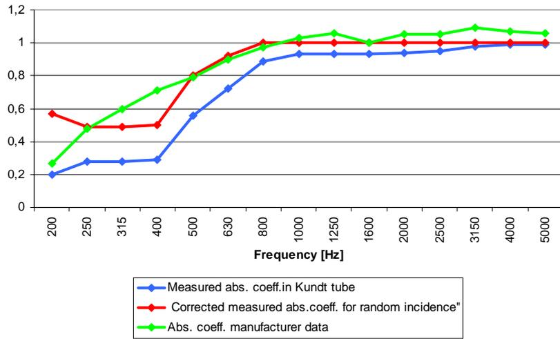
Figure 5: Absorption coefficient of the measured sample using Kundt's tube, and the manufacturer data as reference.
