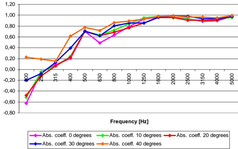
Figure 6: Absorption coefficient measured for various angles of incidence.
