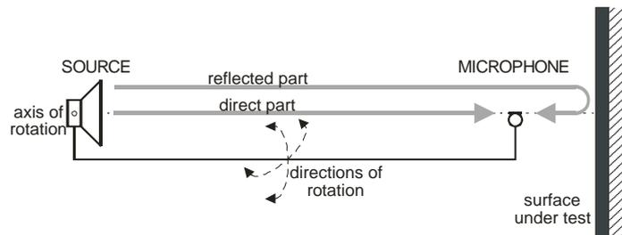
Figure 3: The measurement set-up: the source and the microphone are on a distance of 125 cm, and the microphone is placed 25 cm from the measured surface.
