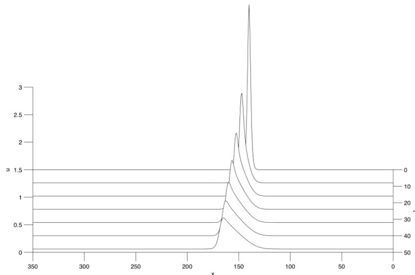
Figura 2. Propagation of a pressure pulse in a nonlinear dispersive media and front formation.
