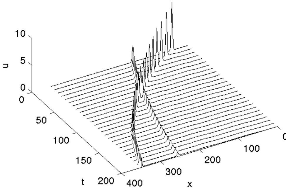
Figura 1. Interaction of two pressure pulses in a nonlinear dissipative and dispersive medium.
