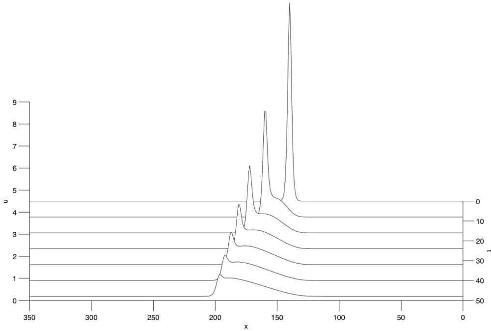
Figura 3. Propagation of a pressure pulse in a nonlinear dispersive media, front formation and tail dissipation.
