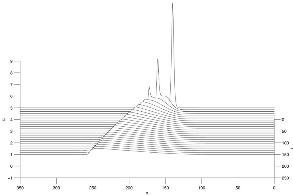
Figura 4. Propagation of a pressure pulse in a nonlinear dispersive media, front formation and tail dissipation.
