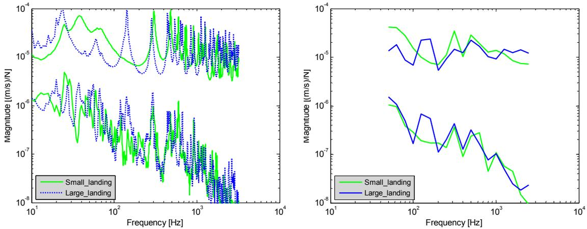
Figure 5: Average transfer mobilities to reference positions of the landings (upper curves) and to the wall (lower curves) in narrow bands and 3rd octave bands
