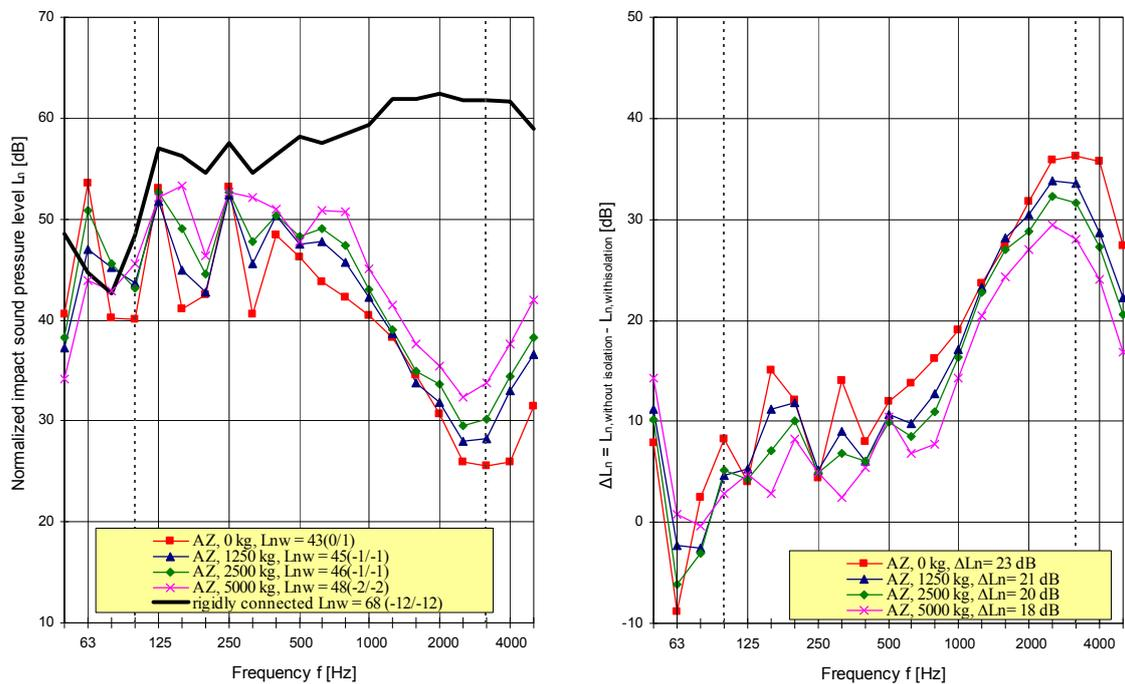
Figure 4: Left: Normalized impact sound pressure level of resiliently supported landing (isolation with Schöck-Tronsole AZ) under different static loads and rigidly connected
