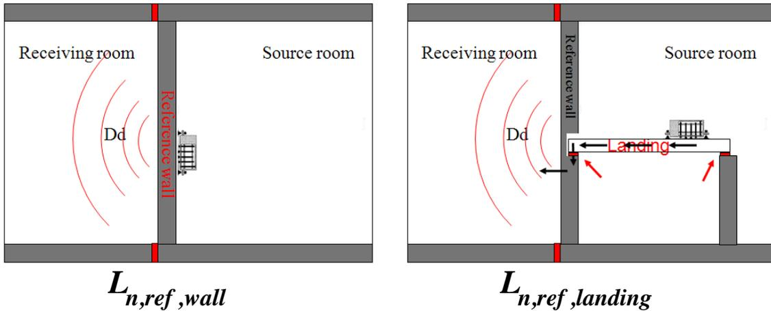
Figure 7: Quantification of the impact-sound reduction of a resiliently supported landing in order to predict the sound transmission in buildings using EN 12354-2 (1). For measurements on the wall an electrodynamic tapping machine with similar force as the standard tpm was used (6).
