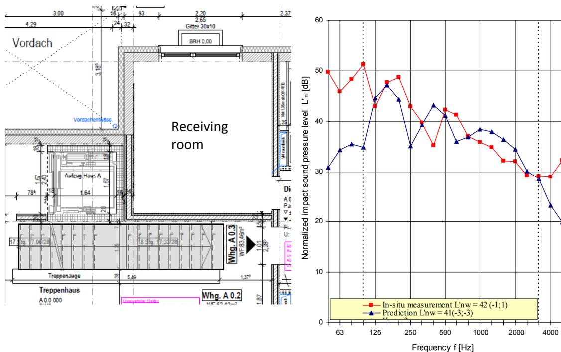
Figure 9: Left: Decoupled flight of stairs in a building situation (5,70 x 1,3 x 0,20 m); stair wall: 24 cm reinforced concrete, density 2300 kg/m<sup>3</sup>; Right: Predicted normalized impact sound pressure level and in-situ measurement
