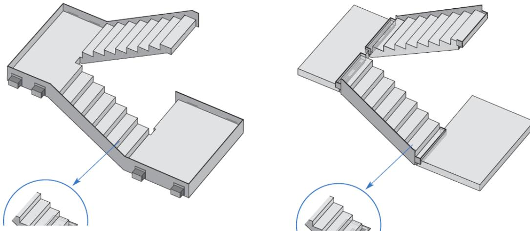
Figure 1: Decoupled stair systems, left: decoupled landings, right: decoupled flight of stairs (pictures provided by manufacturer Schöck Bauteile GmbH)
