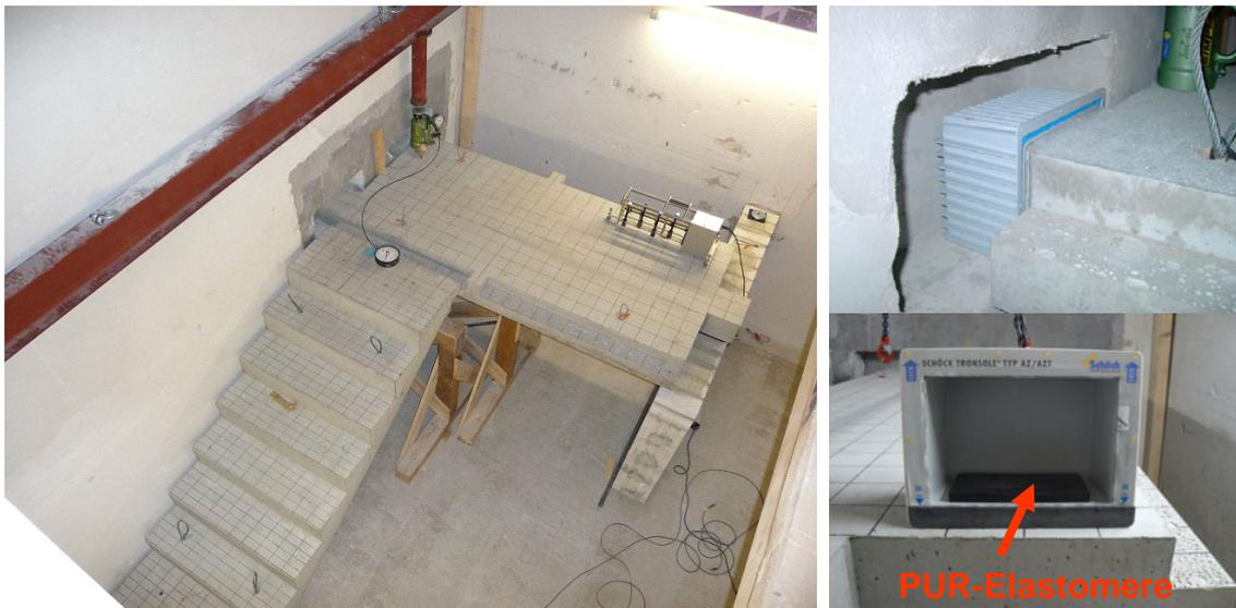
Figure 3: Experimental set-ups to investigate the sound transmission of 1.) resiliently supported landing and 2.) rigidly connected landing and resiliently supported flight of stairs.
