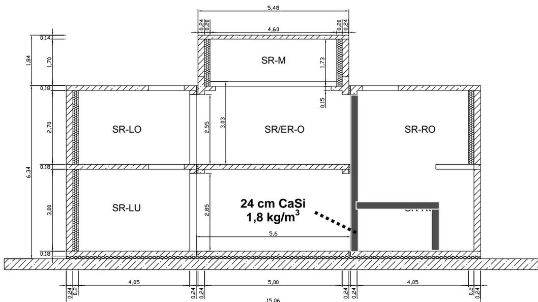
Figure 2: Staircase test facility; stair wall and stair landing indicated in grey
