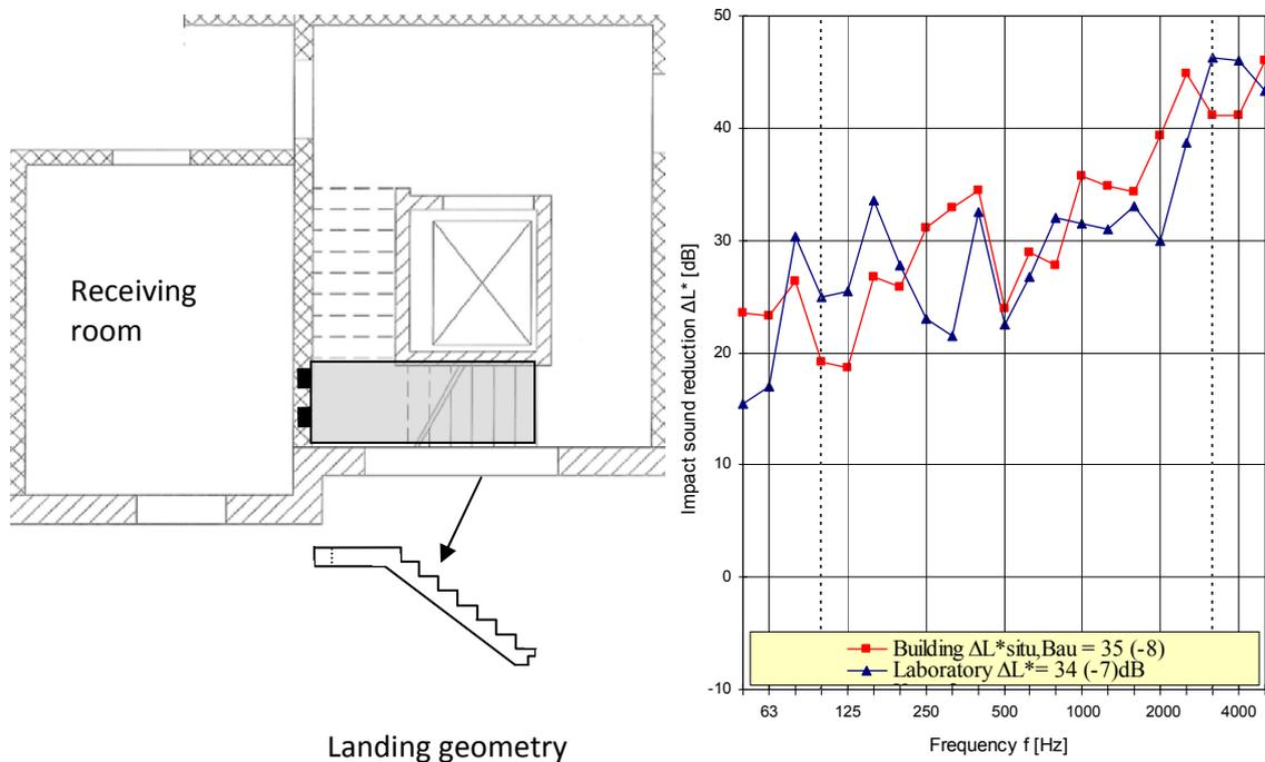
Figure 8: Left: Decoupled stair element in a building situation. Landing (1,0 x 1,0 x 0,18 m) with flight of stairs; stair wall: 24 cm CaSi, density 1800 kg/m<sup>3</sup>; Right: Impact sound reduction according to equation 3 in the building and of the reference landing in the laboratory
