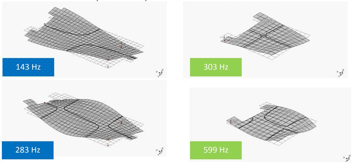
Figure 6: Vibration shapes of a large and a small landing by means of experimental modal analysis
