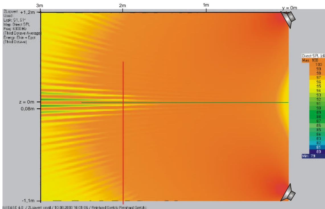
Figure 2: Comb filter effect caused by two elevated loudspeakers (at the right side of the figure), 6300Hz third octave band shown, red/green cursor points to listening position, differences between minima/maxima between 7 and 10 dB, distance between two maxima smaller than 8cm, see z axis on the left side of the figure.
