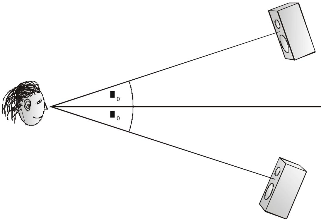
Figure 1: Listening position in preliminary tests, note the symmetric position of the speakers with regard to the listener
