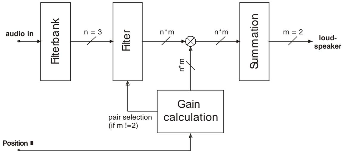
Figure 3: Signal flow graph of elevation panning method, n: number of frequency bands, m: number of elevated loudspeakers for one azimuth direction
