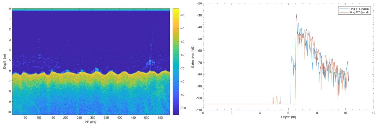
Figure 3 (left): Echogram representation with Matlab® of L1.1 - T5. Above, the original transect, down, the transect with the correction.
