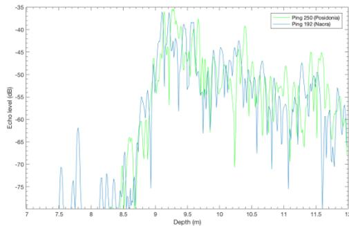
Figure 6 (left): Ping representations of L2.1 – T6 with shells. Blue lines represent pings with a shell and green lines represent pings with only *P. oceanica*.
