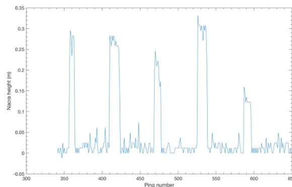
Figure 5: Graphical representation of the height of each shell measured with single pings.
