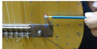
Figure 1: Set-up for modal analysis of the guitar.
