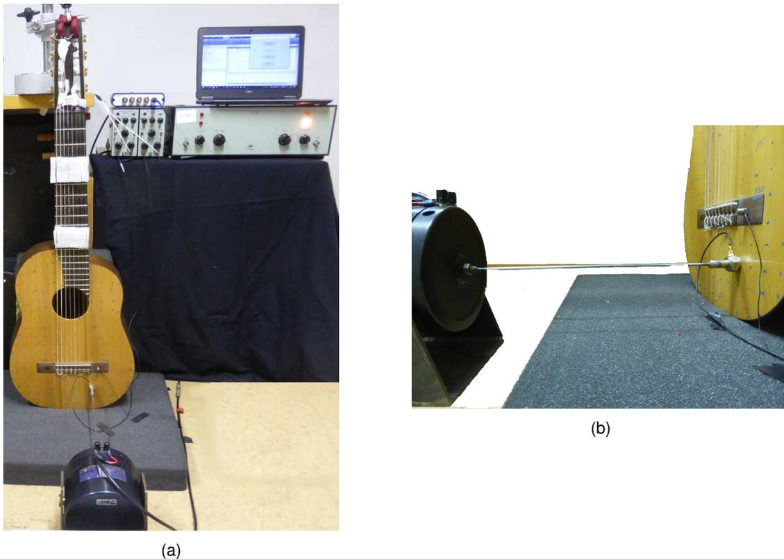
Figure 5: Experimental set-up for vibrating the guitar. (a) Global view with the PC controller, the acquisition module, the amplifier and the shaker; (b) detail of the shaker mounting with the force transducer and accelerometer.
