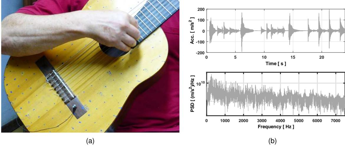
Figure 4: Live playing recording (a) and representative acceleration signal measured at the bridge (b).
