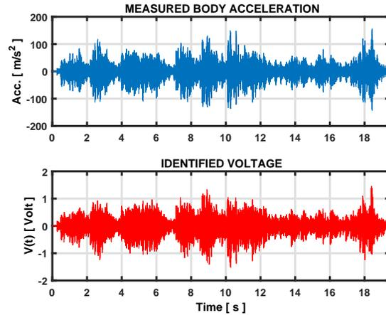
Figure 7: Measured acceleration and identified drive voltage. Opening of *Asturias*.
