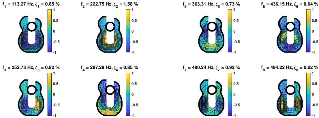
Figure 3: Modal frequencies, modal damping value and mode shape for the principal lower-order modes.
